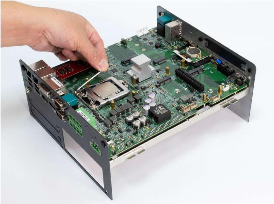
5. Paste thermal pad (1-BRRC60001A1, 29x29x0.8mm) on the CPU.
