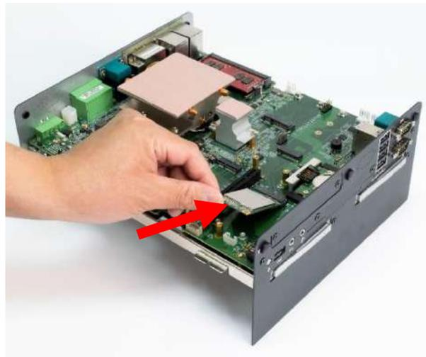
2. Press the Mini PCIe card down and lock it with two screws (M2x3.7L).
