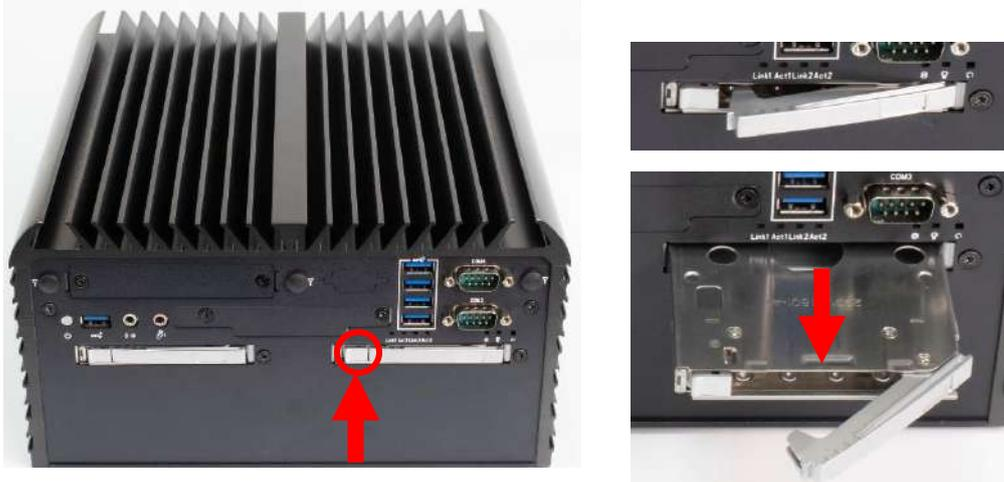
2. Unlock the drive lock (red circle) and insert the HDD/SSD
