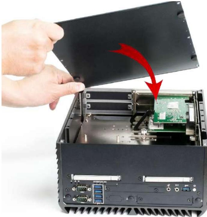
2. Lock the bottom cover with the six screws (M3x5L).
