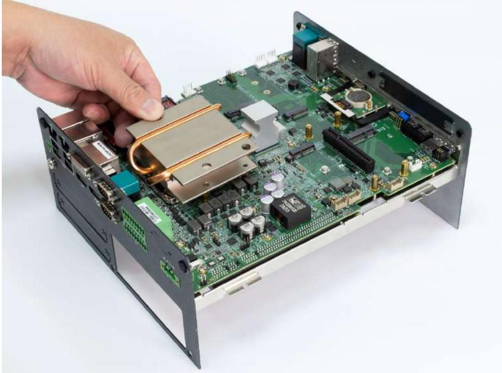
7. Lock the heat block with three screws (M3x5L). Screw driver will be able to penetrate through the holes on the top in order to fasten the screws with copper stud.
