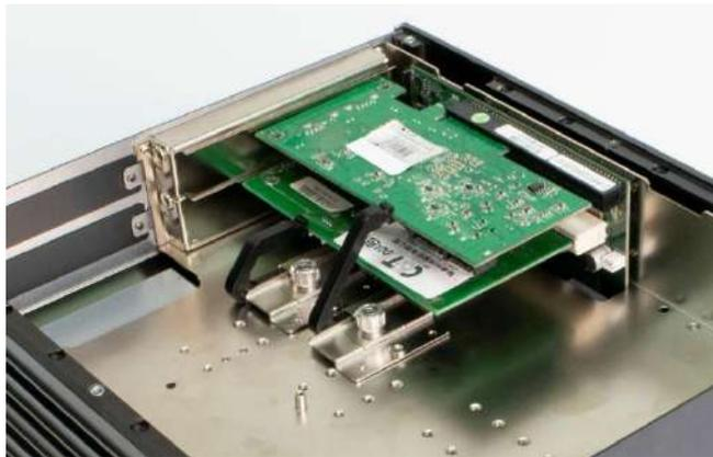
2. Fasten the four screws (M3x5L) below to lock the expansion module.
