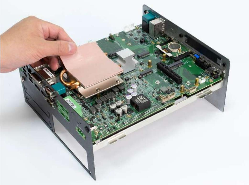
9. Paste the thermal pad (1-BR0500042, 23x20x2.0mm) onto the installed heat block.
