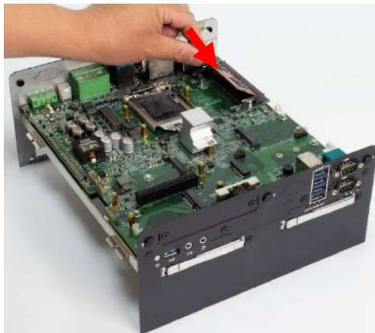
3. Press the memory module vertically downward until you hear the “click” sound. Make sure the memory module is firmly in place.
