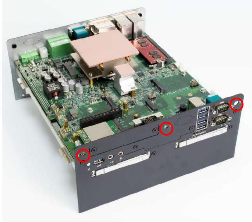
2. Have antenna jack penetrate through the hole, and fasten the nut with SMA jack.
