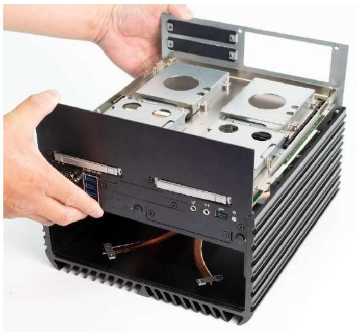
4. Push the system body down until it is firmly in place.
