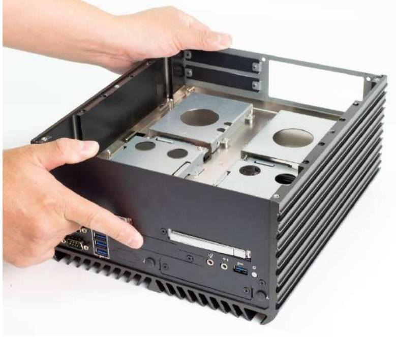
5. Fasten the four screws (M3x5L) to lock the system body with top cover.
