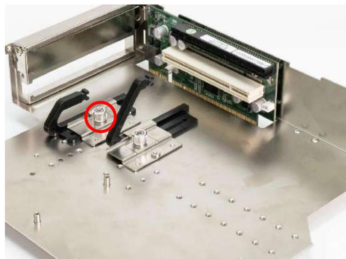
4. Install the PCIe/PCI card according to the below direction and ensure the gold finger is inserted into the slot. Then fasten the screw in the circle.
