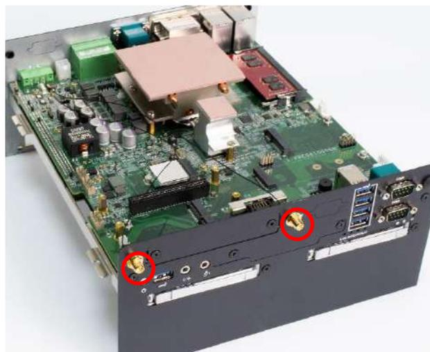
6. Assemble the antenna and SMA jack together.
