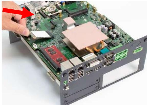
2. Press the Mini PCIe card down and lock it with two screws (M2x3.7L).
