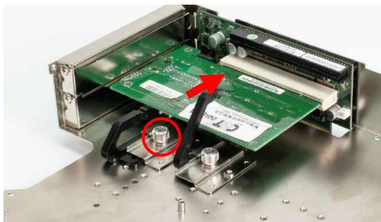
5. Adjust the arm until it holds the card firmly in place. Then fasten the sun screw on the holder.
