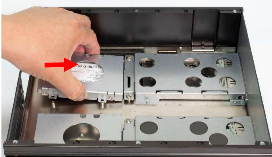
5. Fasten the four screws to lock the internal HDD/SSD bracket.
