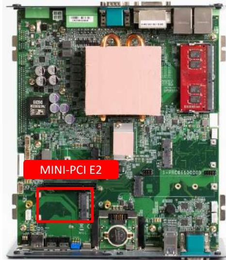
1. Insert Mini PCIe card from 45 degree direction.
