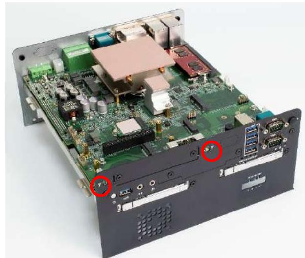
5. Have antenna jack penetrate through the hole, and fasten the nut with SMA jack.
