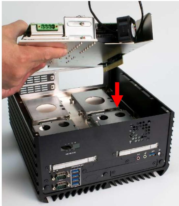
2. Fasten the four screws (M3x5L) below to lock the expansion module.
