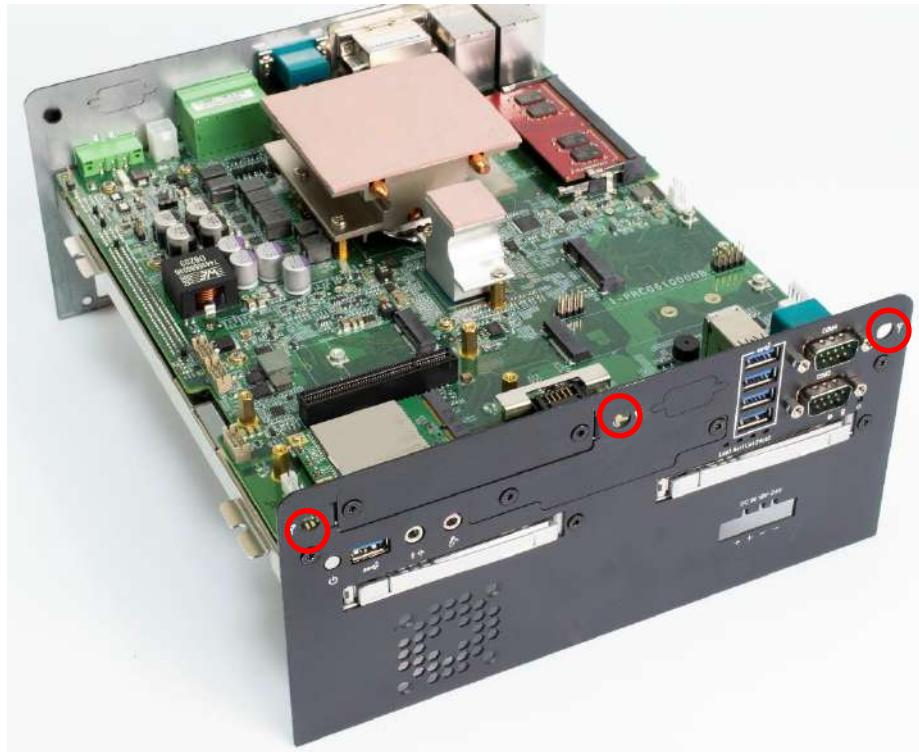
2. Have antenna jack penetrate through the hole, and fasten the nut with SMA jack.
