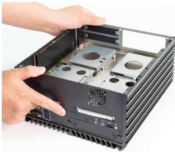
4. Fasten the four screws (M3x5L) to lock the system body with top cover.
