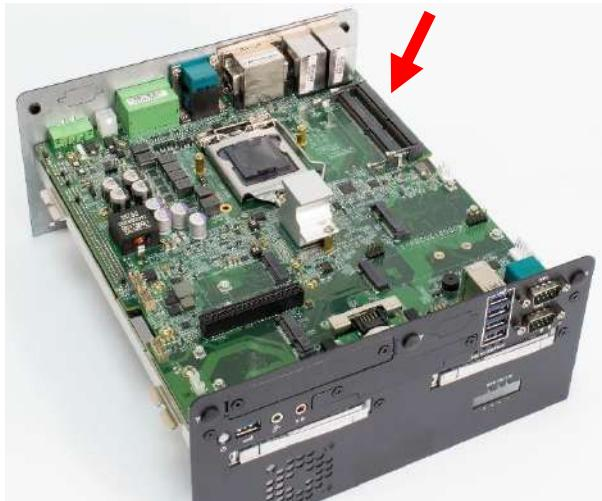
2. Insert memory module from 45 degree direction.
