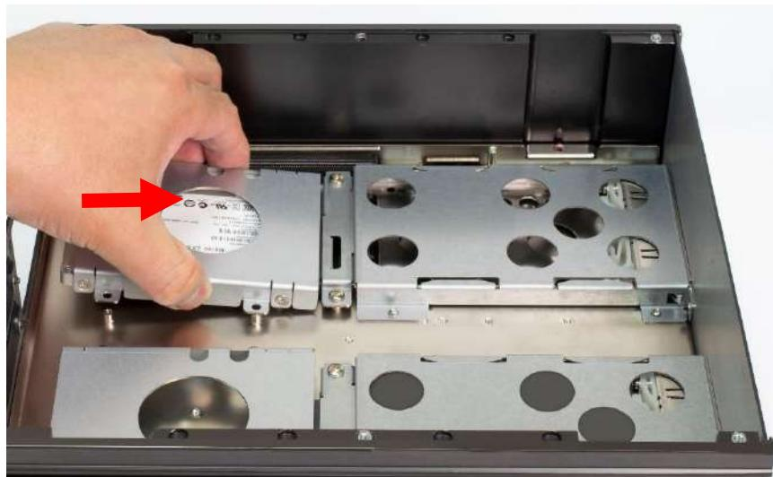
5. Fasten the four screws to lock the internal HDD/SSD bracket.
