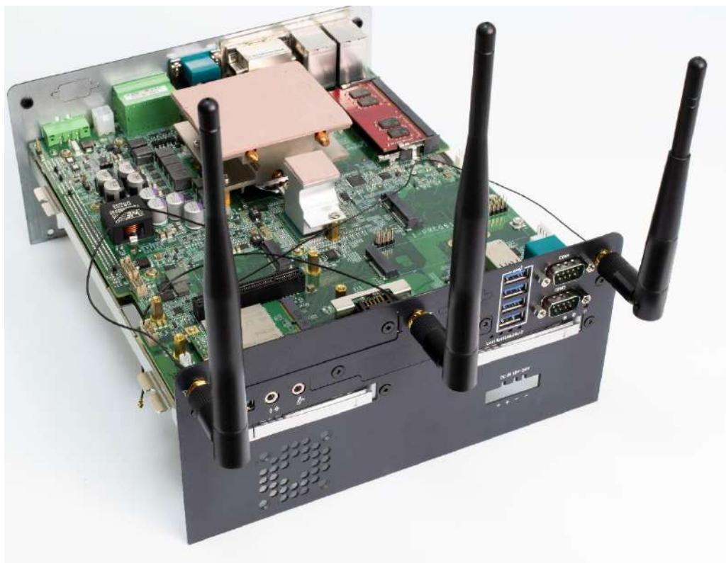
4. Attach the RF connector at the cable-end onto the communication module.
