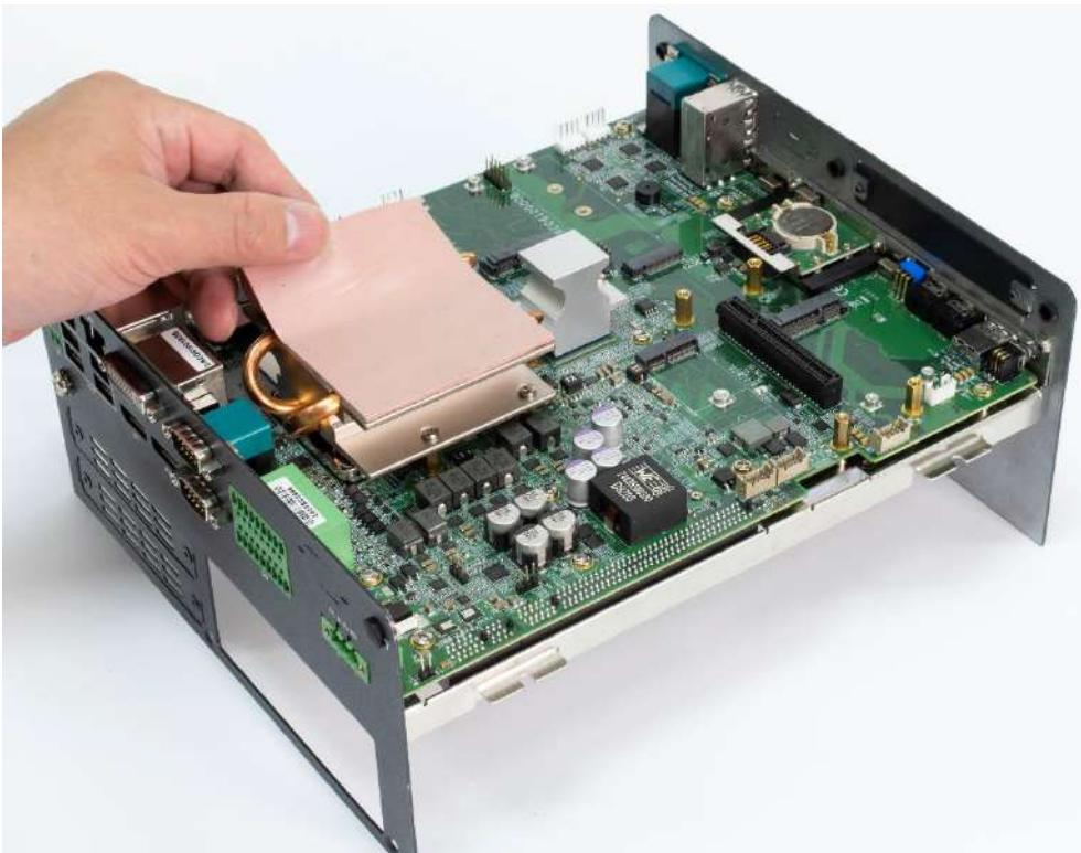
9. Paste the thermal pad (1-BR0500042, 23x20x2.0mm) onto the installed heat block.
