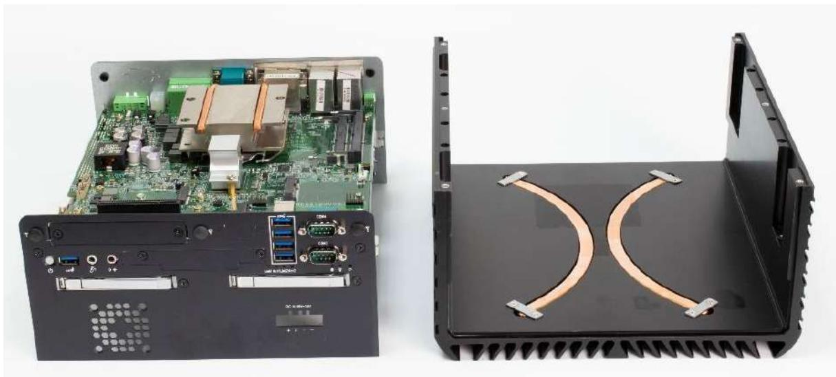
2. Ensure thermal pad is in place on both the CPU and PCH thermal block.
