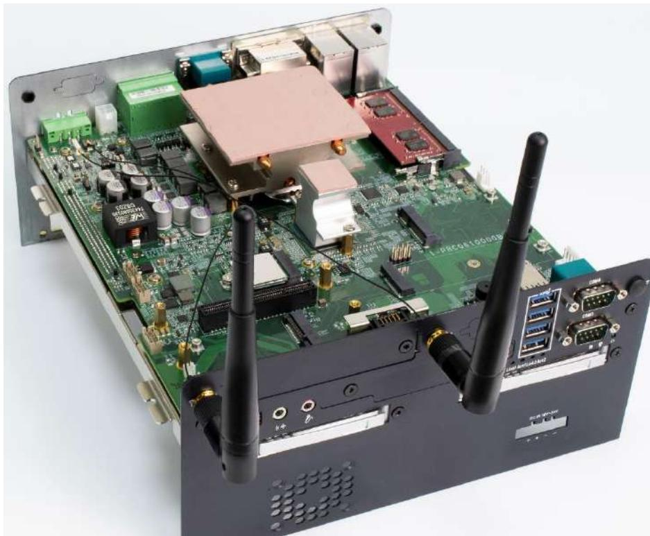
7. Attach the RF connector at the cable-end onto the communication module.
