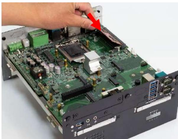
3. Press the memory module vertically downward until you hear the “click” sound. Make sure the memory module is firmly in place.
