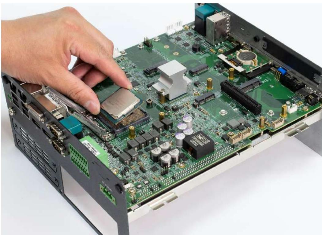
4. Press down the lever again to hold the socket cover.
