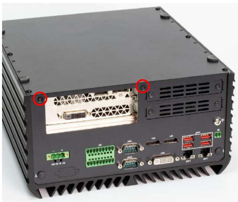
4. Remove the four screws (M3x5L) in the circle below, for the fan ( M3x5L )
