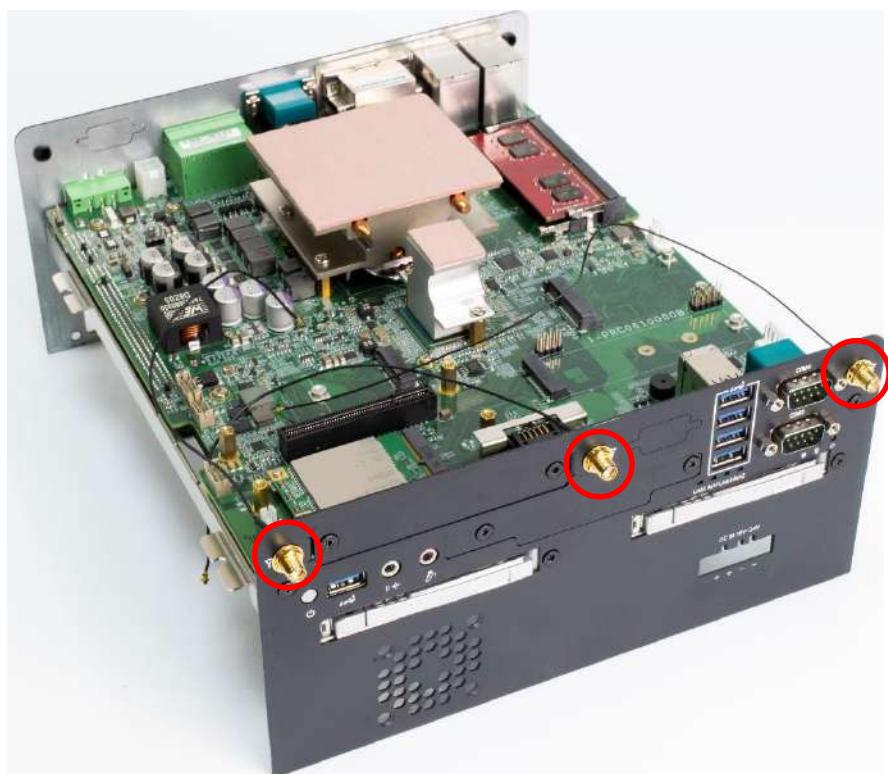
3. Assemble the antenna and SMA jack together.
