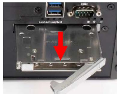
2. Unlock the drive lock (red circle) and insert the HDD/SSD
