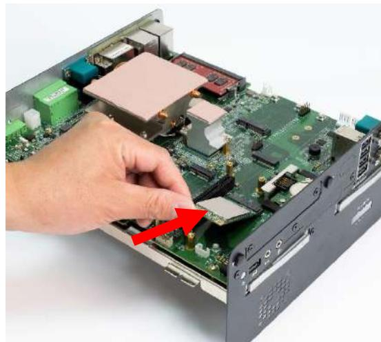
2. Press the Mini PCIe card down and lock it with two screws (M2x3.7L).
