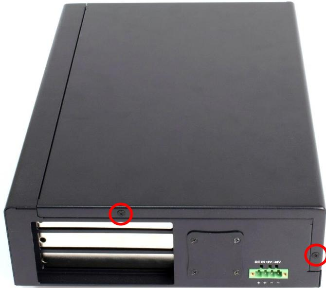
2. Push the chassis cover following the below direction to open the expansion module.
