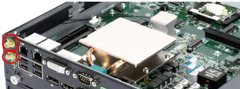
**5. Assemble the antenna and SMA jack together.**
