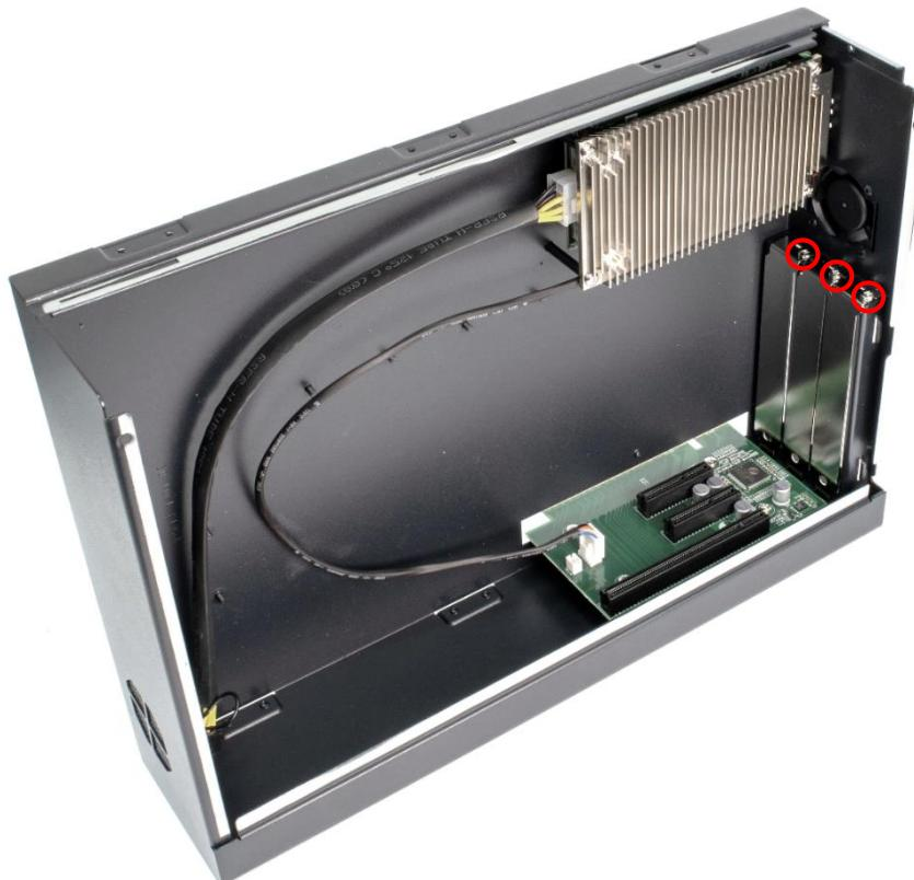
**10. Install the graphic card according to the below direction and ensure the gold finger is inserted into the slot. and then fasten the screws.**
