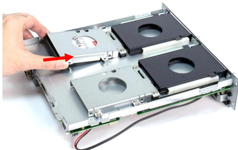
**5. Fasten the 4 screws to lock the internal HDD/SSD bracket.**
