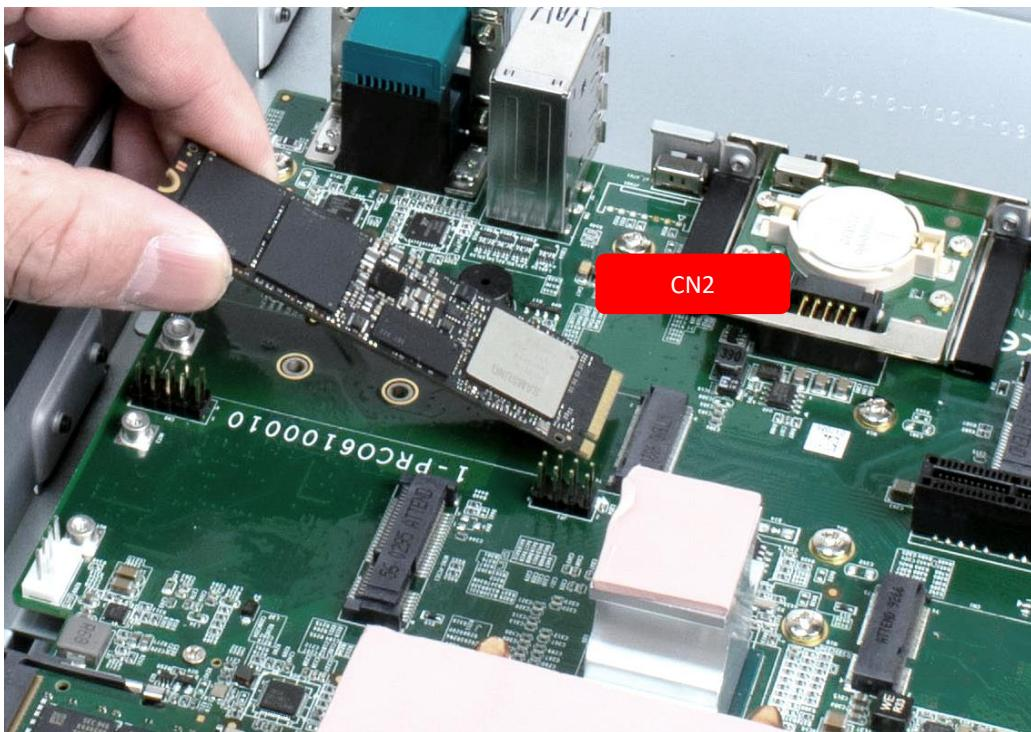
2. Press the M.2 M Key card down and lock it with one screw (M2x3.7L).
