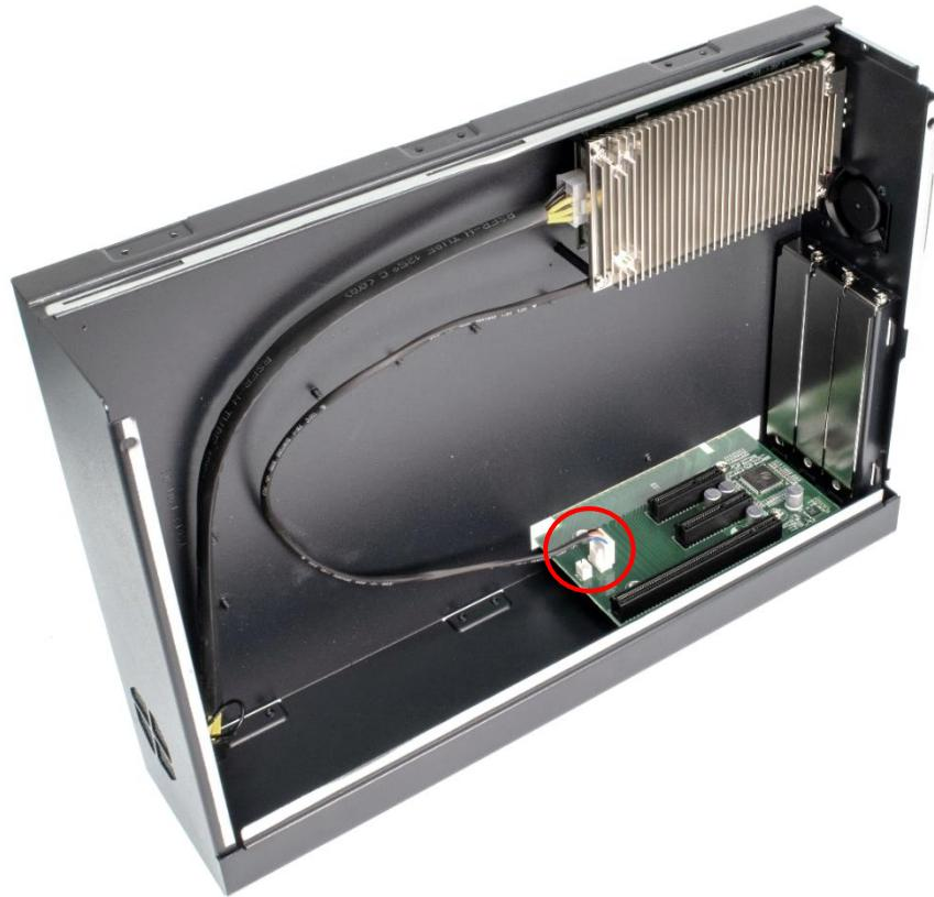
**9. Unscrew the card bracket screws to remove the bracket from the expansion slots.**
