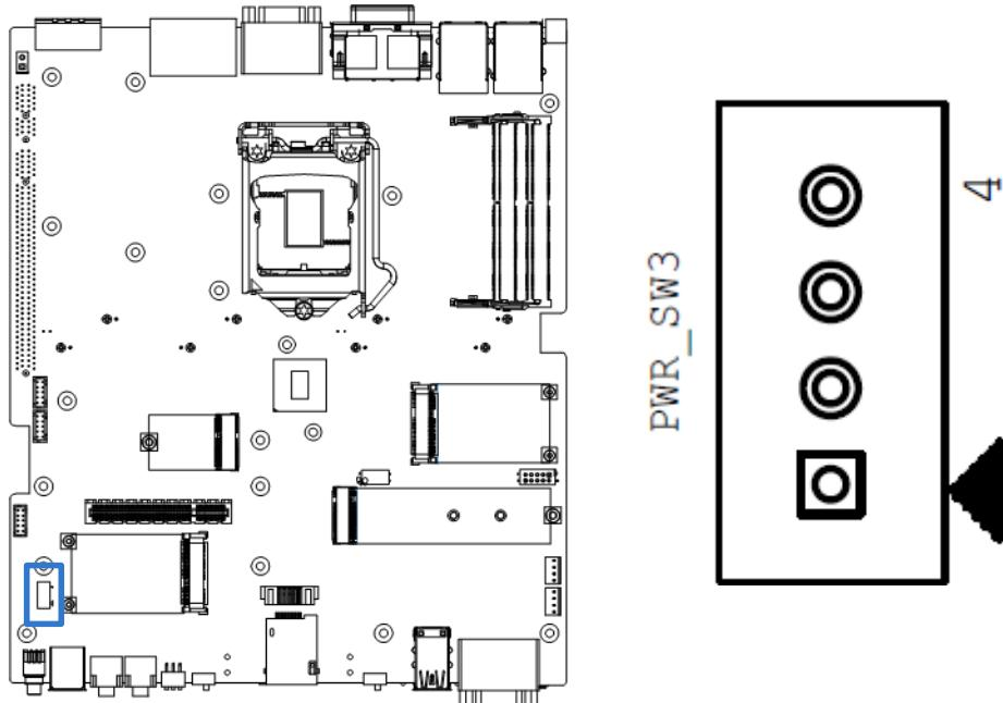
PWR\_SW3 : Remote Power Switch 1x4 pin box header, 2.0mm pitch
