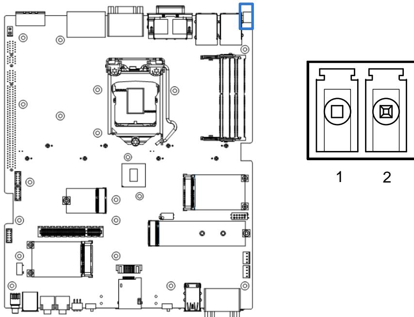
PWR\_SW2 : Remote Power Switch Type: Terminal Block 1x2 2-pin, 3.5mm pitch
