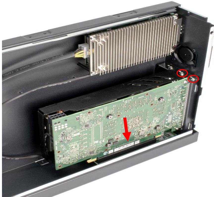
**11. Adjust the arm until it holds the card firmly in place.**
