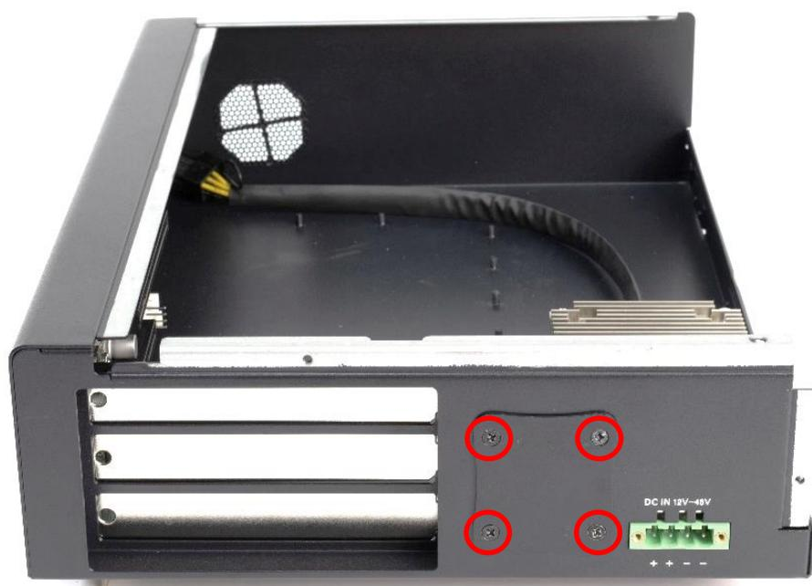
**6. Install the fan according to the below direction**
