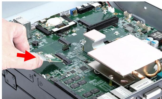
2. Press the Mini PCIe card down and lock it with two screws (M2x3.7L).
