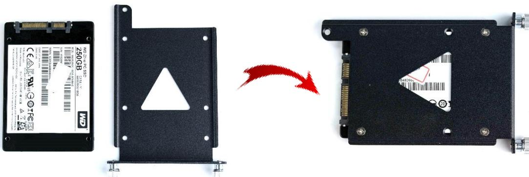
**3. Slide the HDD bracket back and then fasten the sun screws.**
