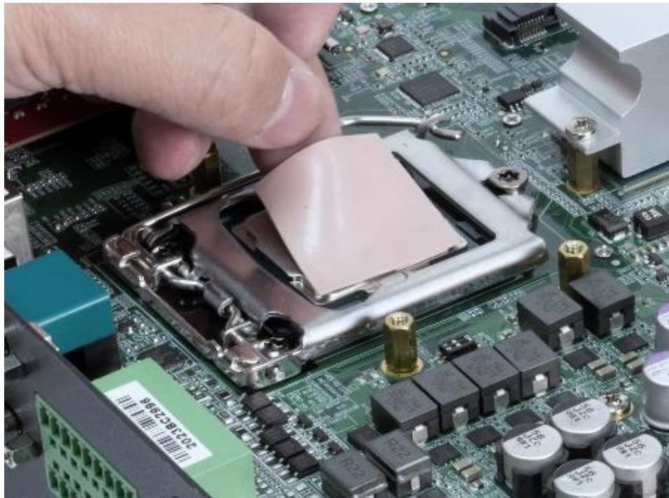
**6. Place the designated heat block onto the CPU with thermal pad.**
