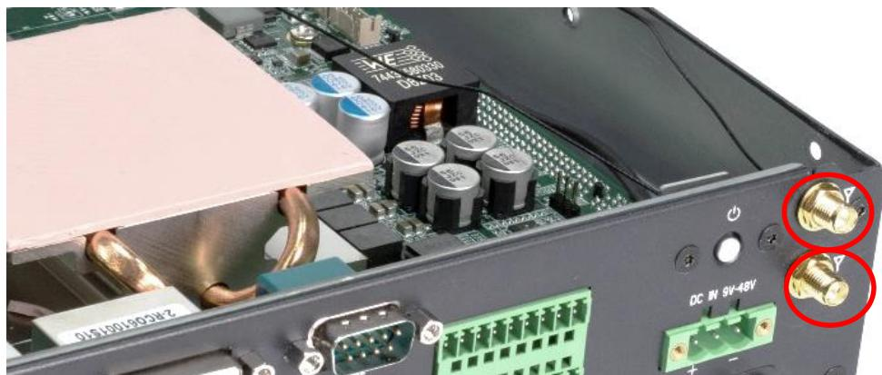
**3. Assemble the antenna and SMA jack together.**
