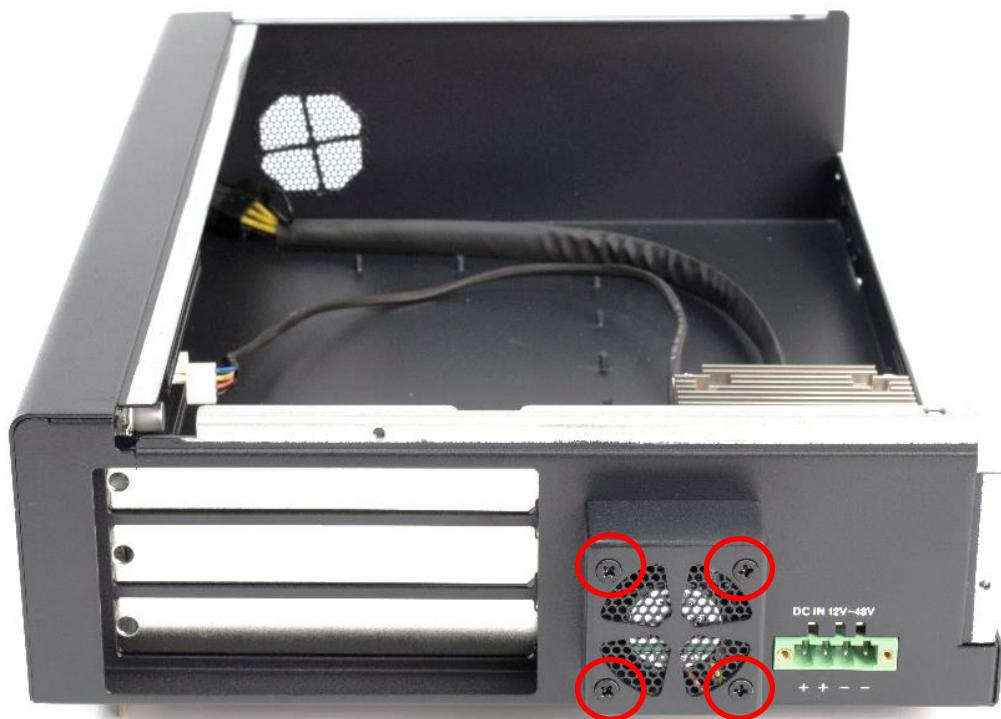
**8. Insert fan power cable**
