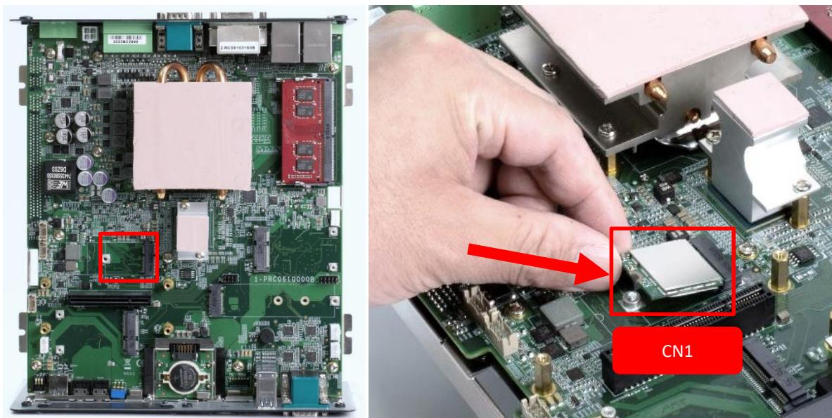
2. Press the M.2 E Key card down and lock it with one screw (M2x3.7L).
