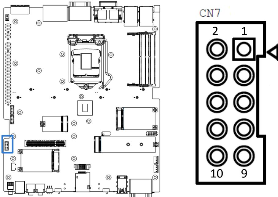
**CN7 : USB2.0 Connector 2x5 10-pin box header, 2.0mm pitch**
