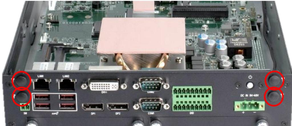
**4. Have antenna jack penetrate through the hole, and fasten the nut with SMA jack.**
