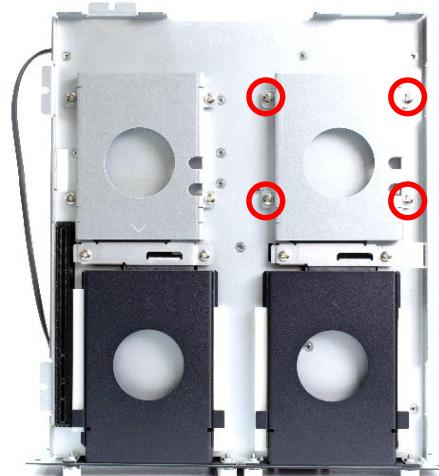
3. Lock the 2.5" HDD with HDD/SSD bracket using four screws (M3x4L).
