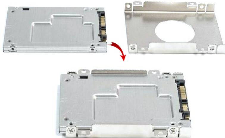
**4. Install the HDD/SSD bracket following the direction below.**
