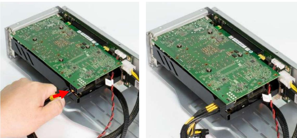
14. Adjust the arm until it holds the card firmly in place.
