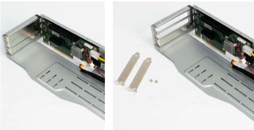
11. Install the graphic card according to the below direction and ensure the gold finger is inserted into the slot.
