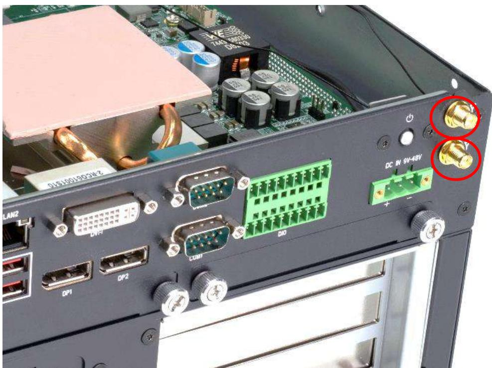
3. Assemble the antenna and SMA jack together.
