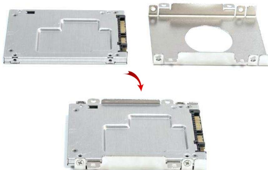
4. Install the HDD/SSD bracket following the direction below.
