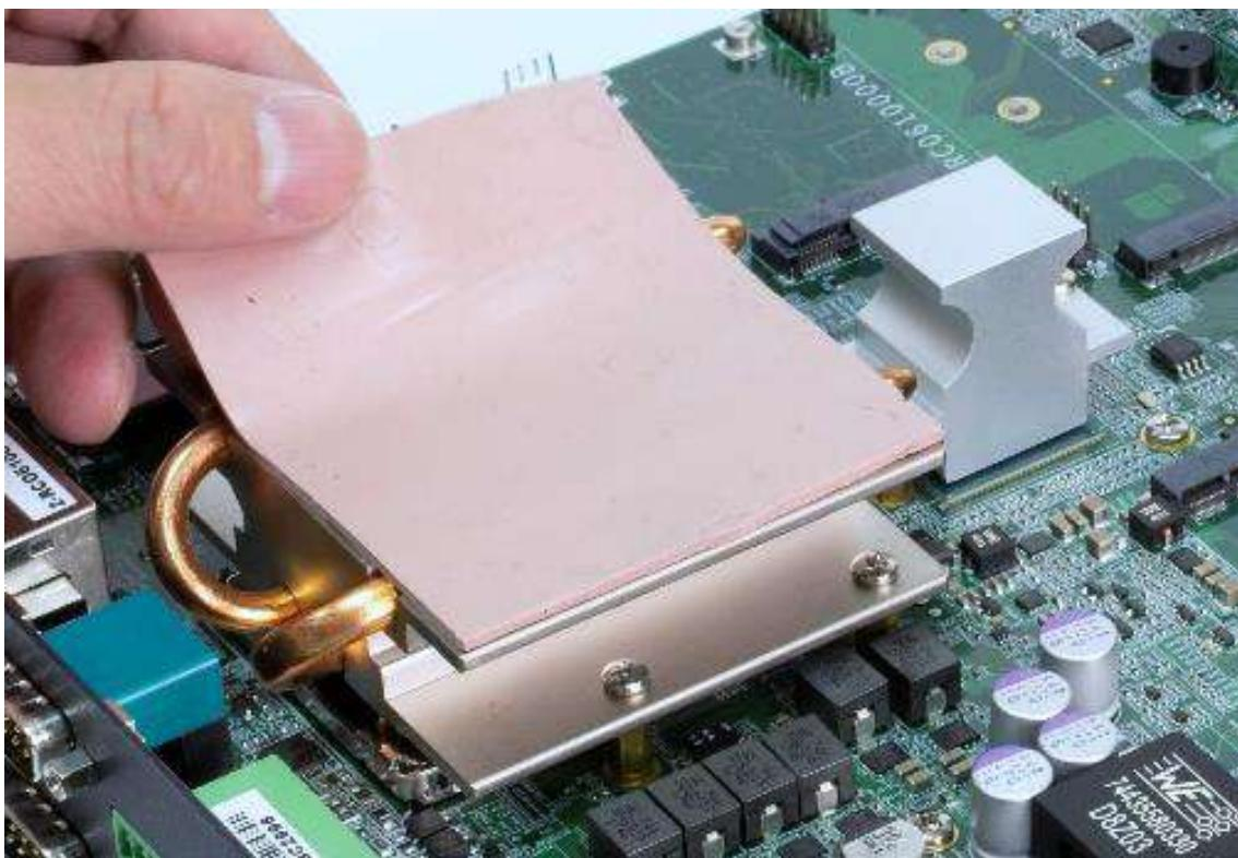
9. Paste the thermal pad onto the installed heat block.
