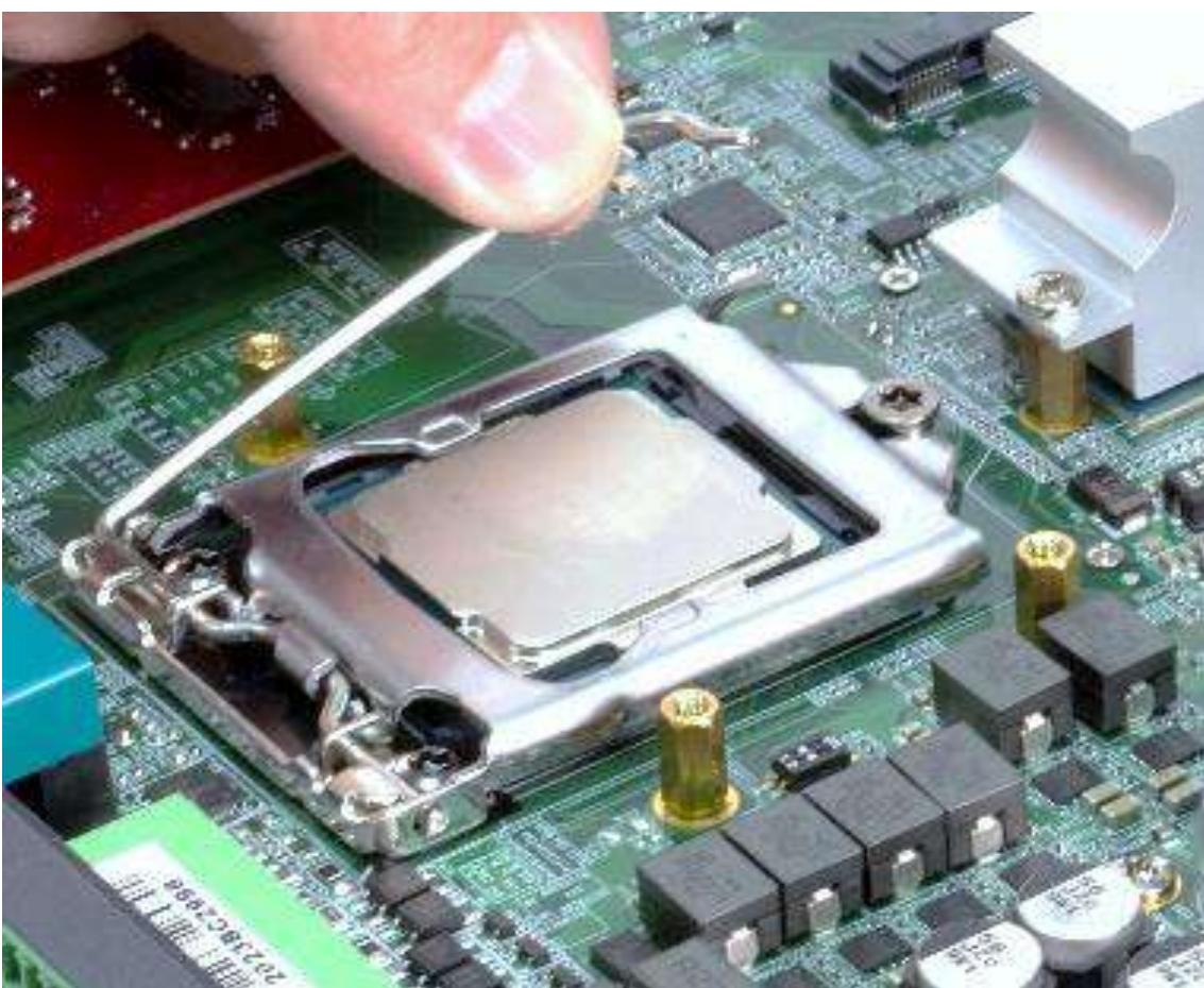
5. Paste thermal pad on the CPU.
