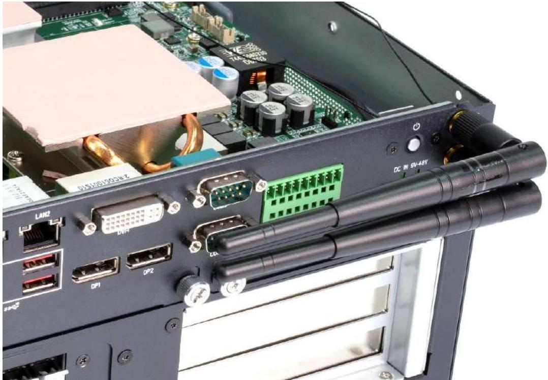
4. Attach the RF connector at the cable-end onto the communication module.
