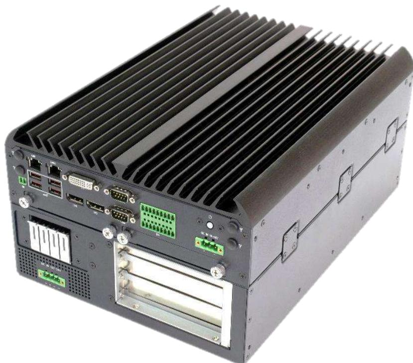
1. Unscrew the 4 screws on the top side of computing module
