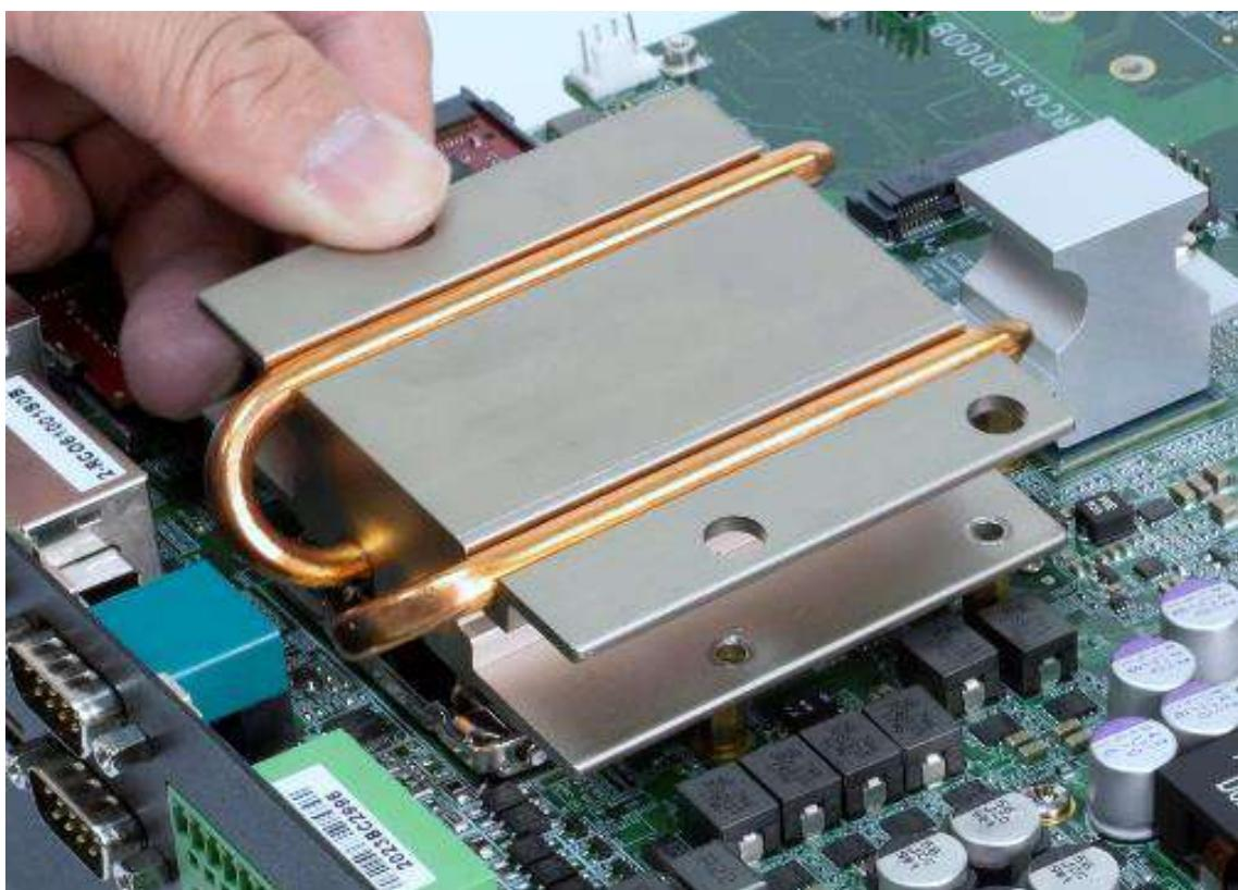
7. Lock the heat block with three screws (M3x5L). Screw driver will able to penetrate through the holes on the top in order to fasten the screws with copper stud.
