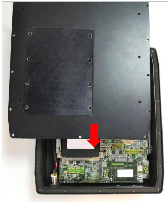
2. Lock the bottom cover with the eighteen screws.
