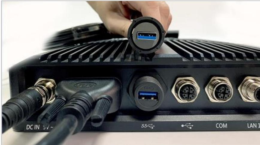
5. Install external M12 A-CODE 8P USB 2.0 cable. Please align the foolproof opening and tighten the locking ring to secure waterproof cable.
