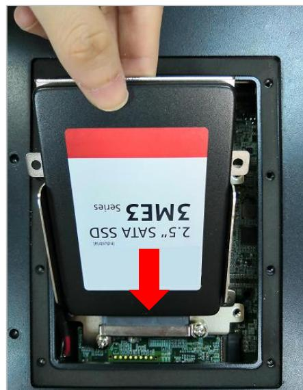
4. Fasten the four screws to lock the internal SATA HDD bracket.
