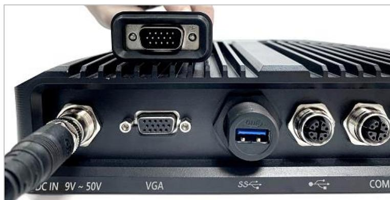
4. Install external waterproof USB 3.0 cable. Please align the foolproof opening and tighten the locking ring to secure waterproof cable.
