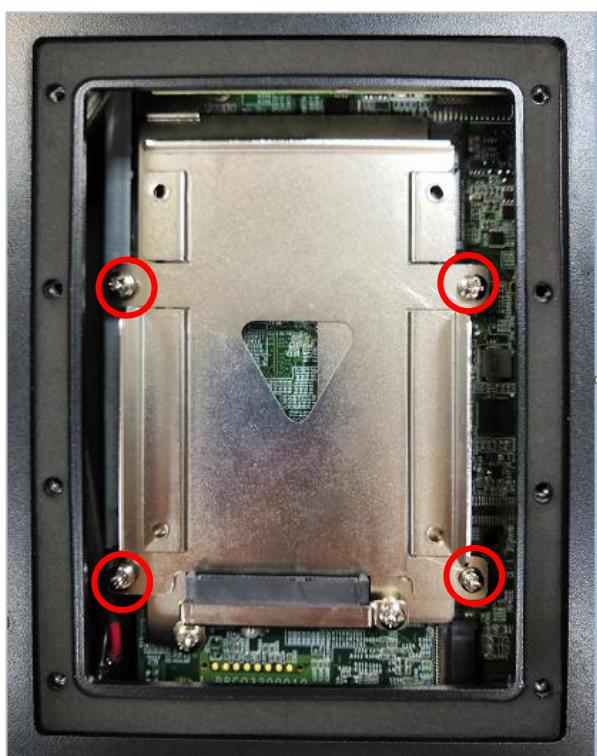
3. After removing internal SATA HDD bracket, you will be able to access the memory slot.
