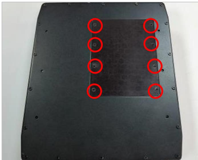
2. Unscrew the below four screws to remove the internal SATA HDD bracket.
