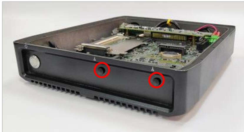
2. Remove antenna hole cover on the system panel.
