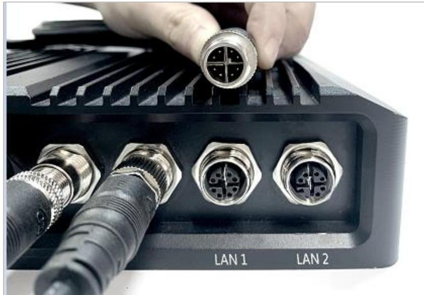
8. Install external M12 X-CODE 8P LAN2 cable. Please align the foolproof opening and tighten the locking ring to secure waterproof cable.
