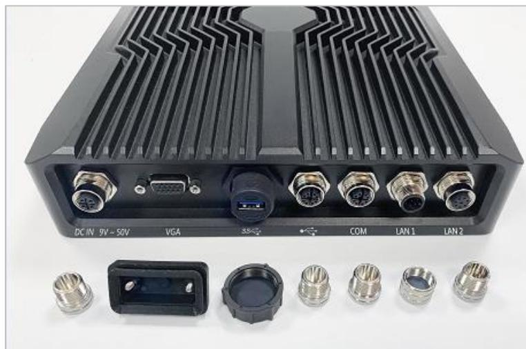
2. Install external M12 A-CODE 4P power cable. Please align the foolproof opening and tighten the locking ring to secure waterproof cable.
