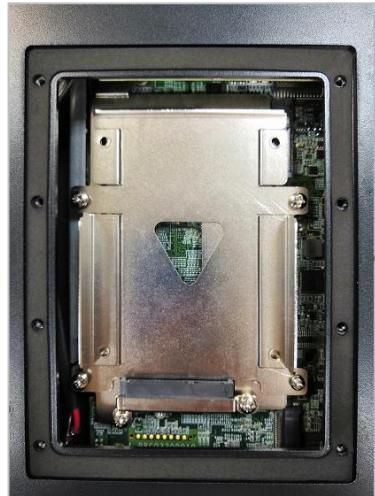
2. Lock the 2.5" HDD with HDD bracket using four screws (M3x4L).
