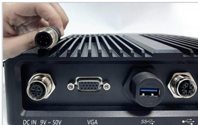
3. Install external waterproof VGA cable. Please align the connector direction and tighten the locking ring to secure waterproof cable.
