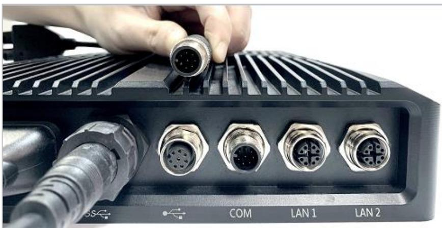
6. Install external M12 A-CODE 8P COM cable. Please align the foolproof opening and tighten the locking ring to secure waterproof cable.
