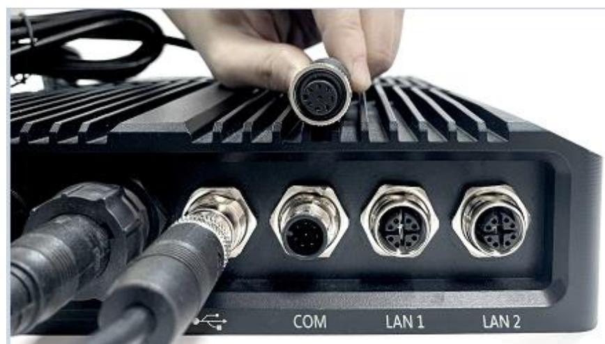
7. Install external M12 X-CODE 8P LAN1 cable. Please align the foolproof opening and tighten the locking ring to secure waterproof cable.
