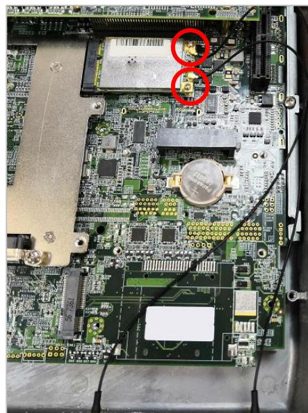
6. Assemble the antenna and antenna jack together.
