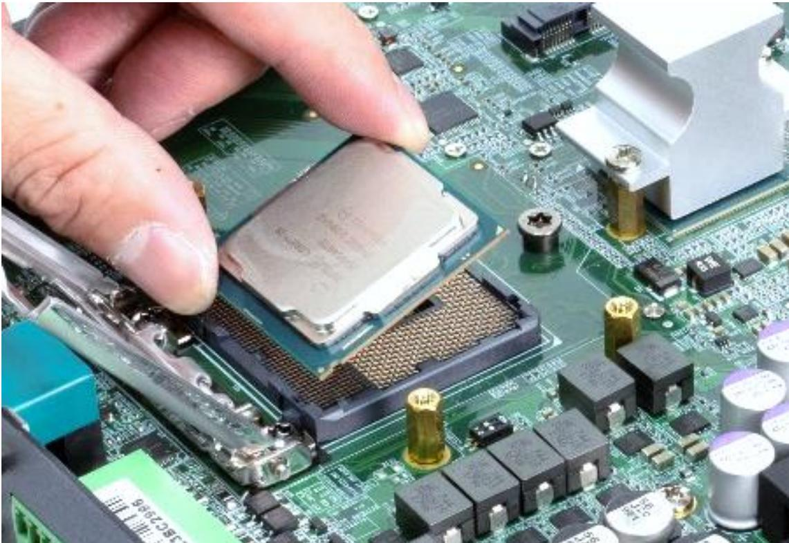
4. Press down the lever again to hold the socket cover.
