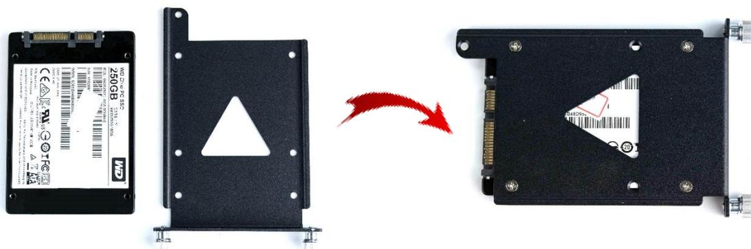
3. Slide the HDD bracket back and then fasten the sun screws.
