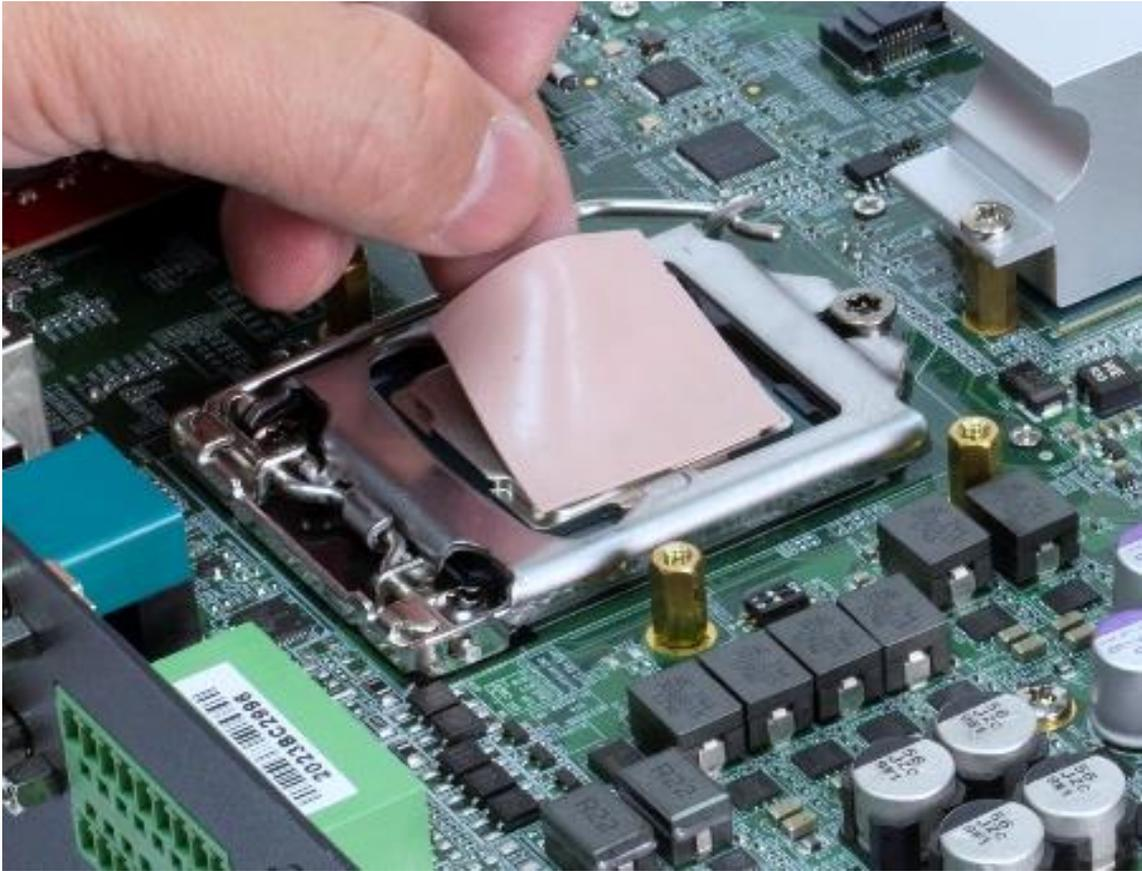
6. Place the designated heat block onto the CPU with thermal pad.
