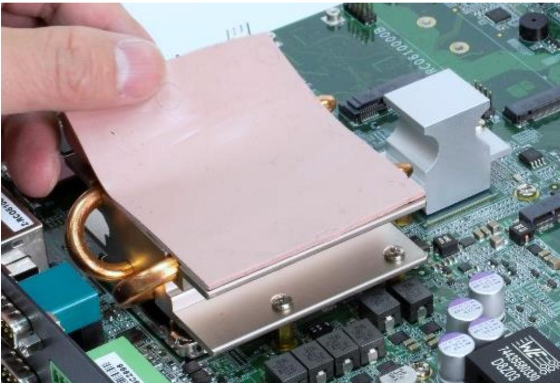
9. Paste the thermal pad onto the installed heat block.
