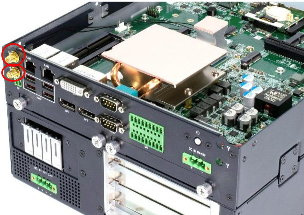
5. Assemble the antenna and SMA jack together.
