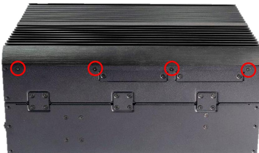
2. Unscrew the 4 screws on the bottom side.
