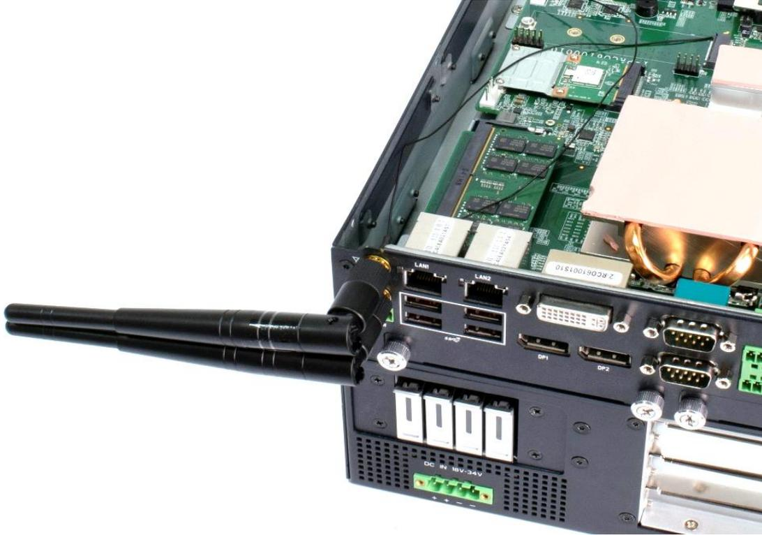
6. Attach the RF connector at the cable-end onto the communication module.
