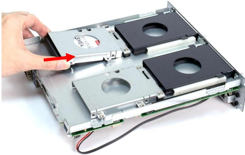
5. Fasten the 4 screws to lock the internal HDD/SSD bracket.
