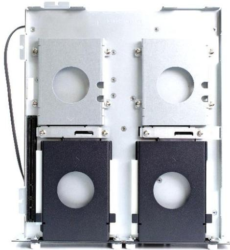
2. Unscrew the 4 screws (M3x5L) to remove the internal SATA HDD/SSD bay.
