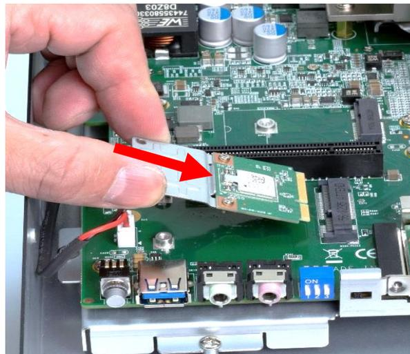
2. Press the Mini PCIe card down and lock it with two screws (M2x3.7L).
