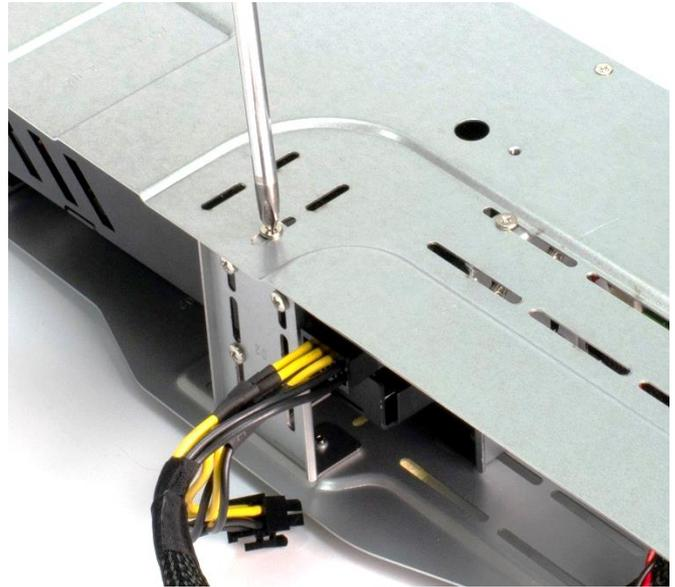
18. Put the graphic expansion module into the expansion chassis.
