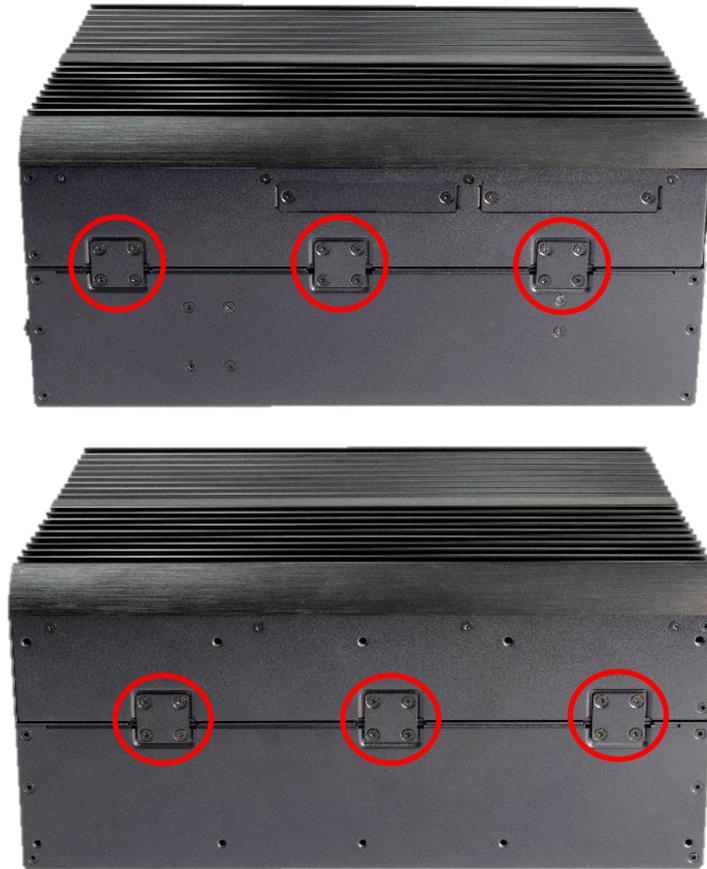
2. Now you can separate the expansion module from the computing module.
