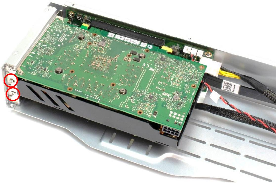
13. Insert power cable from the power board to the graphic card.
