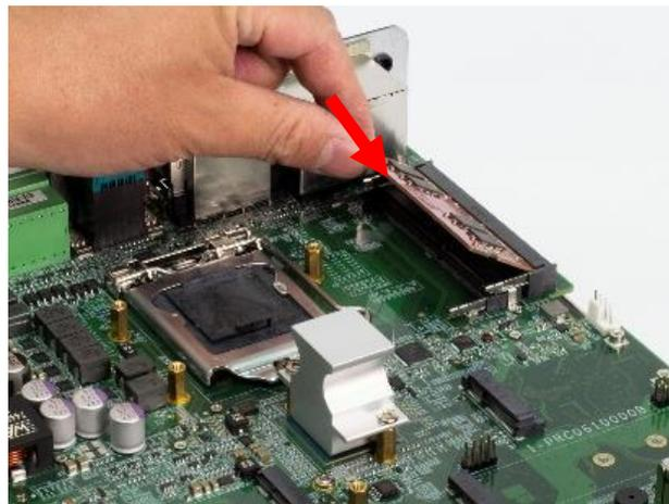
3. Press the memory module vertically downward until you hear the "click" sound. Make sure the memory module is firmly in place.
