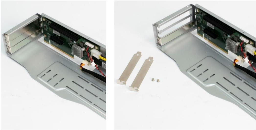
11. Install the graphic card according to the below direction and ensure the gold finger is inserted into the slot.
