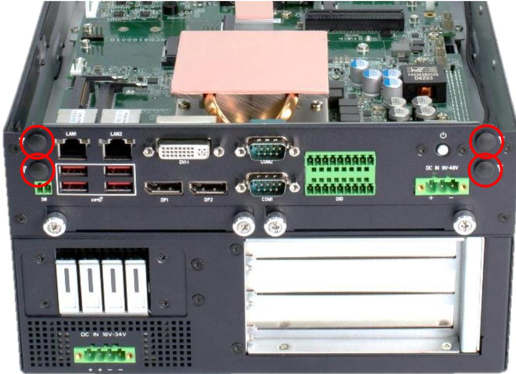
4. Have antenna jack penetrate through the hole, and fasten the nut with SMA jack.
