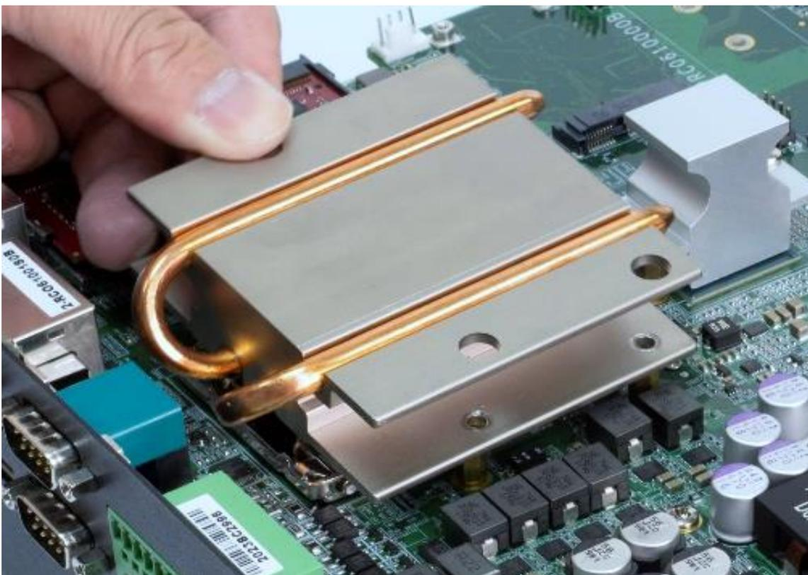
7. Lock the heat block with three screws (M3x5L). Screw driver will be able to penetrate through the holes on the top in order to fasten the screws with copper stud.
