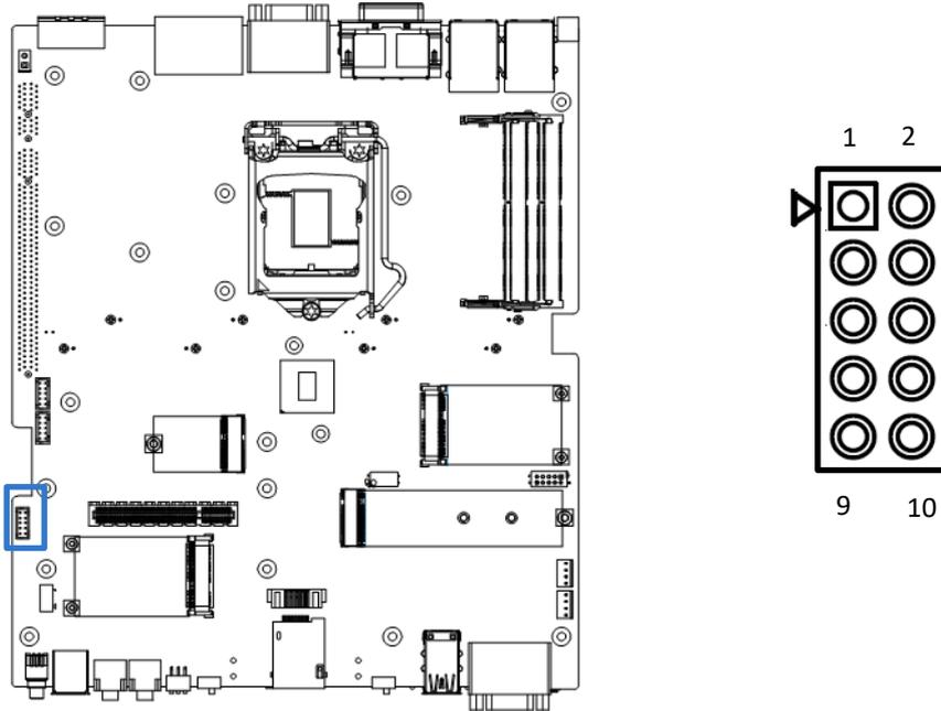
**CN7 : USB3.0 Connector 2x5 9-pin header, 2.0mm pitch**
