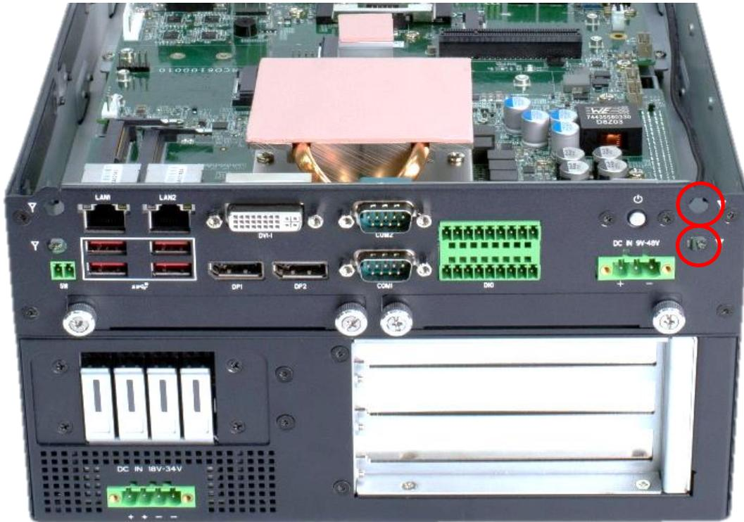
2. Have antenna jack penetrate through the hole, and fasten the nut with SMA jack
