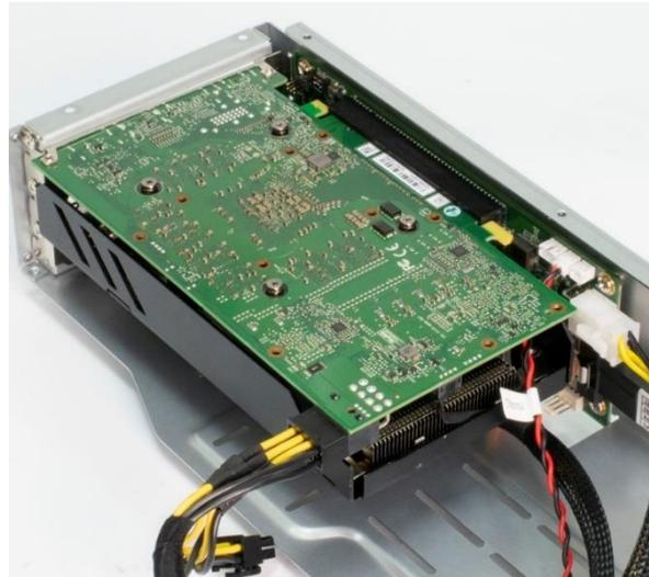
14. Adjust the arm until it holds the card firmly in place.
