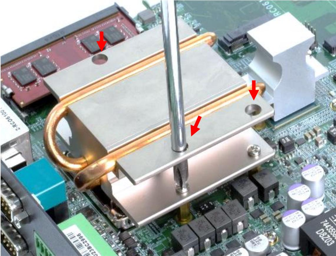
8. Paste the thermal pad onto the installed heat block.
