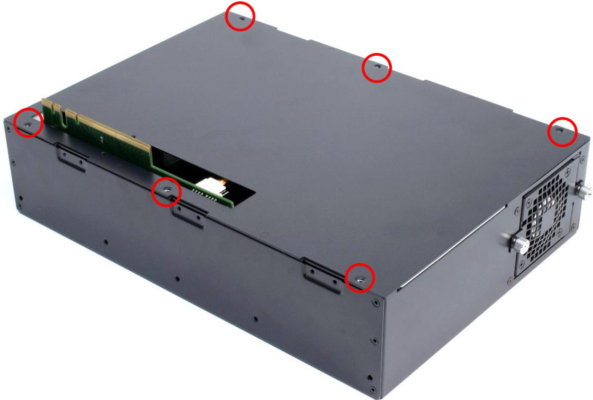
2. Push the chassis cover following the below direction to open the expansion module.
