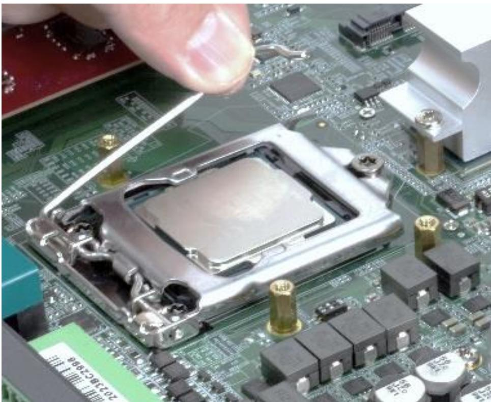
**5. Paste thermal pad on the CPU.**
