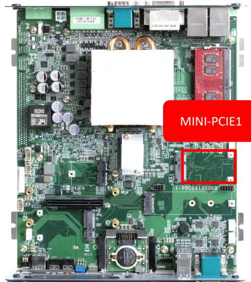
1. Insert Mini PCIe card from 45 degree direction.
