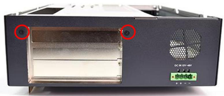
**4. Unscrew the 2 screws to remove the I/O shield.**
