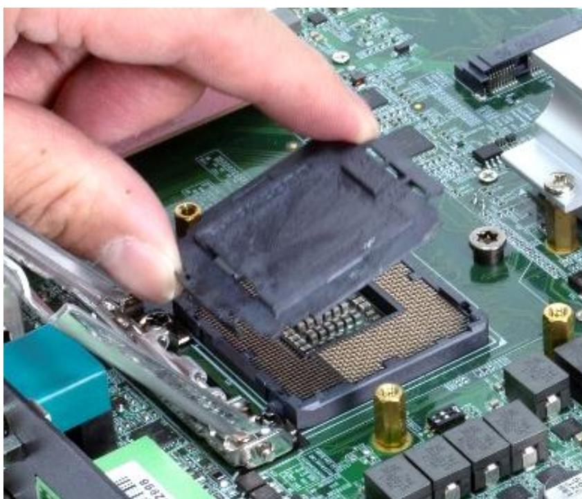
**3. Insert CPU gently.**
