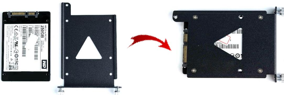
**3. Slide the HDD bracket back and then fasten the sun screws.**
