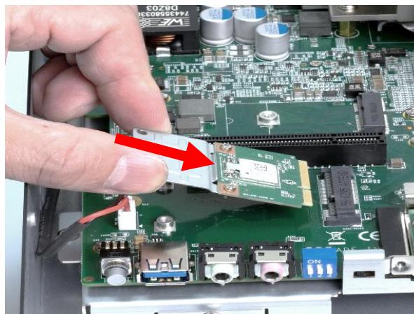
**2. Press the Mini PCIe card down and lock it with two screws (M2x3.7L).**
