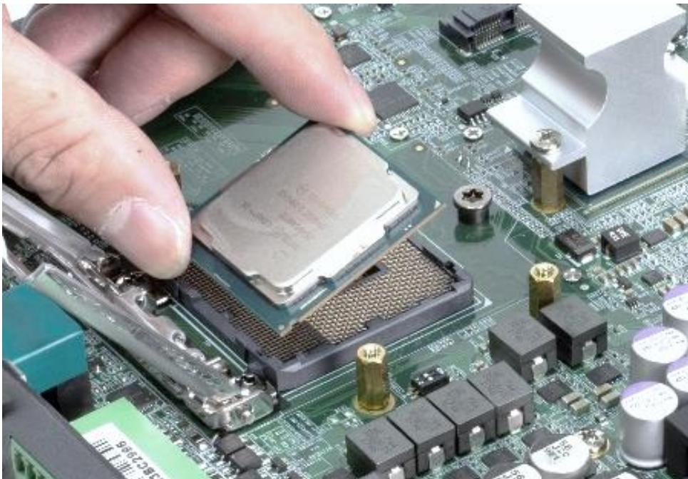
**4. Press down the lever again to hold the socket cover.**
