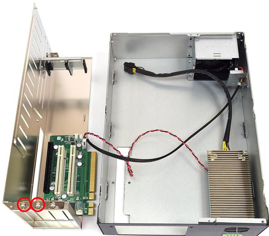
**5. Unscrew the card bracket screws to remove the bracket from the expansion slots.**
