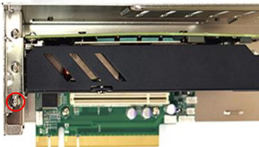
2. Install the PCIe/PCI extension card and ensure the gold finger is inserted into the slot. and then fasten the screw.
