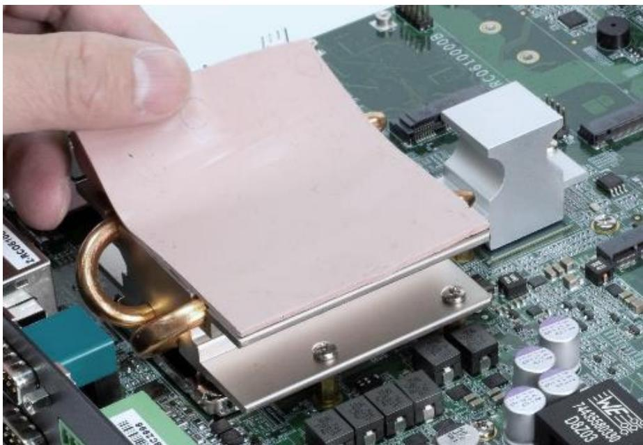
**9. Paste the thermal pad onto the installed heat block.**
