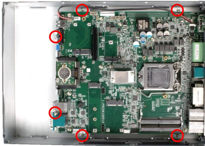
2. Unscrew 4 screws on the front side.
