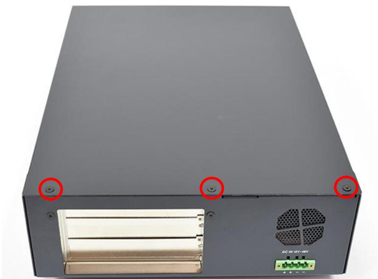
2. Push the chassis cover following the below direction to open the expansion module.
