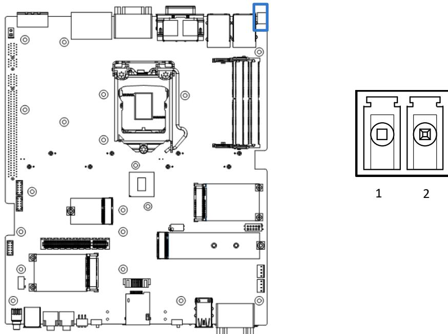
PWR\_SW2 : Remote Power Switch Type: Terminal Block 1x2 2-pin, 3.5mm pitch
