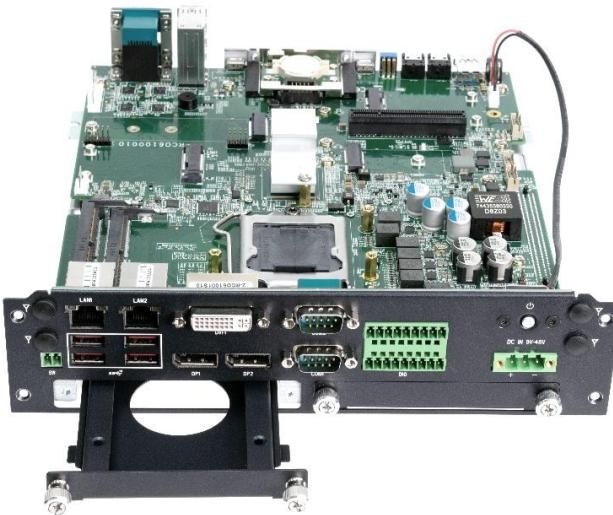
2. Lock the 2.5" HDD with HDD bracket using 4 screws.
