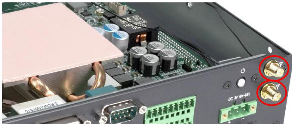
**3. Assemble the antenna and SMA jack together.**
