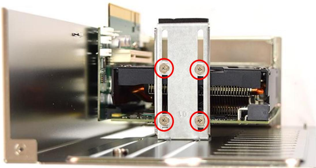
**8. Fasten the 2 screws**
