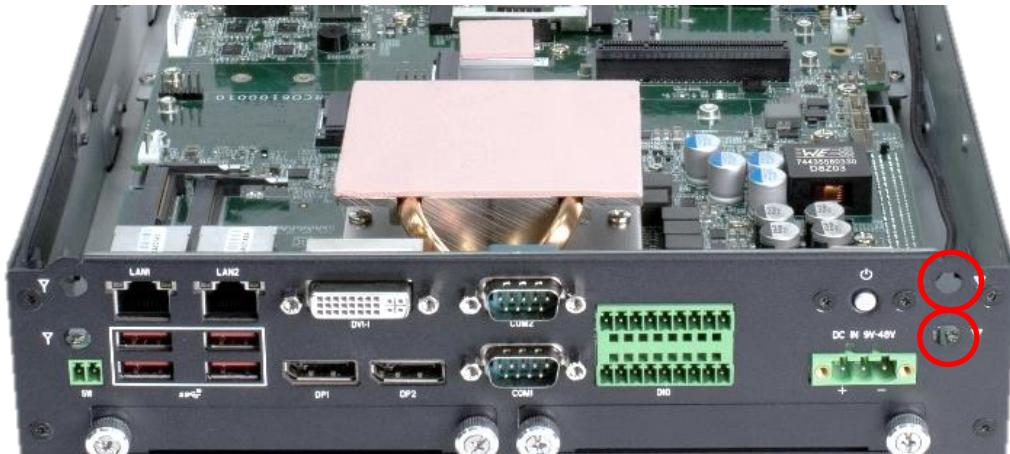
2. Have antenna jack penetrate through the hole, and fasten the nut with SMA jack
