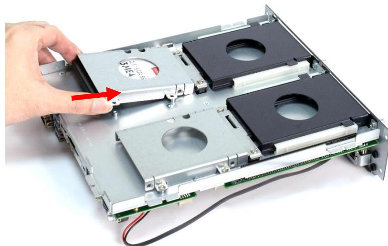
**5. Fasten the 4 screws to lock the internal HDD/SSD bracket.**
