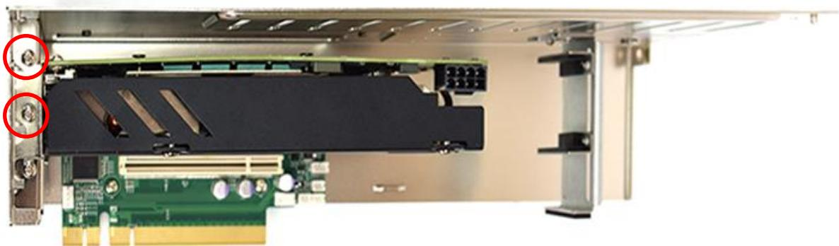
**7. Adjust the arm until it holds the card firmly in place. Then fasten the screw on the holder**
