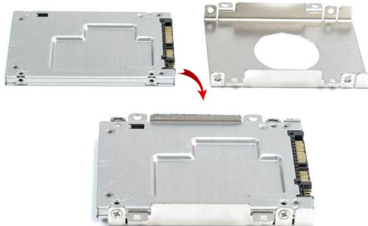
**4. Install the HDD/SSD bracket following the direction below.**
