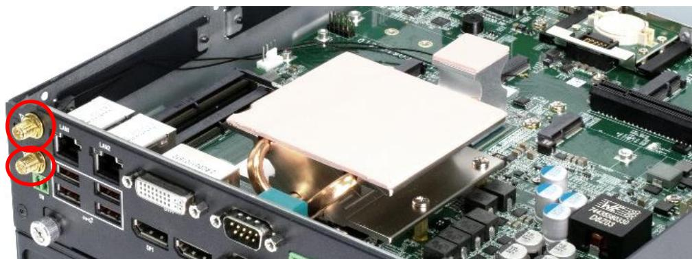
**5. Assemble the antenna and SMA jack together.**
