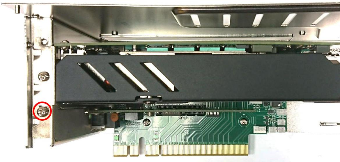
**3. Put the graphic expansion module into the expansion chassis.**
