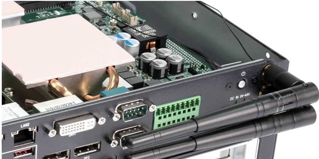
**4. Attach the RF connector at the cable-end onto the communication module.**
