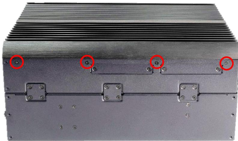
**2. Unscrew the 4 screws on the bottom side.**
