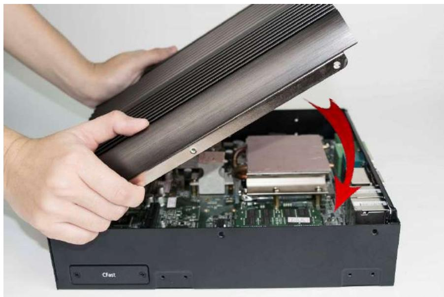
3. Fasten the six screws on the system top side and bottom side.
