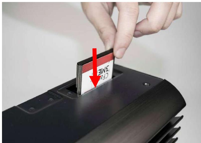
3. The socket is push-push type. Push the installed CFast card again to remove it.
