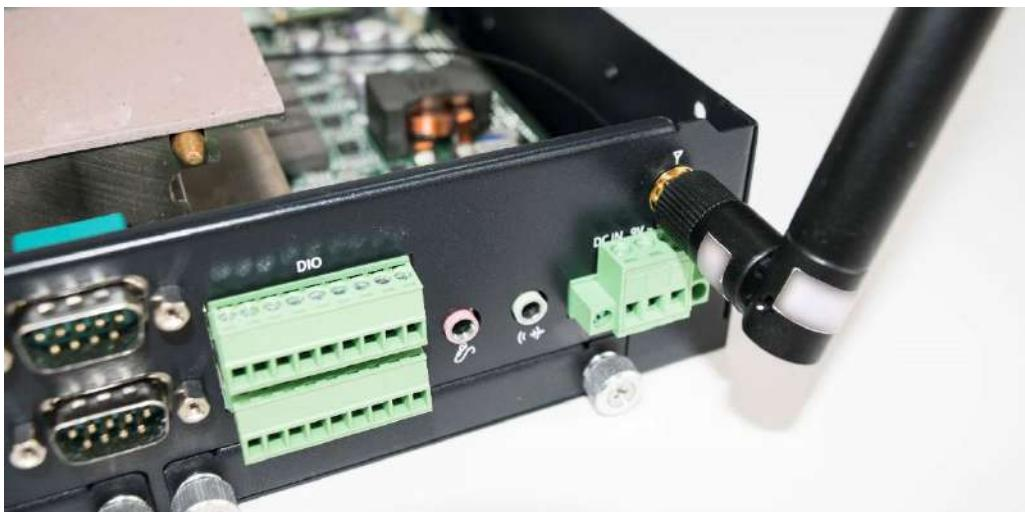
6. Attach the RF connector at the cable-end onto the communication module.
