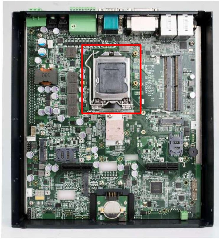
2. Press down the CPU socket lever in order to open the socket cover.
