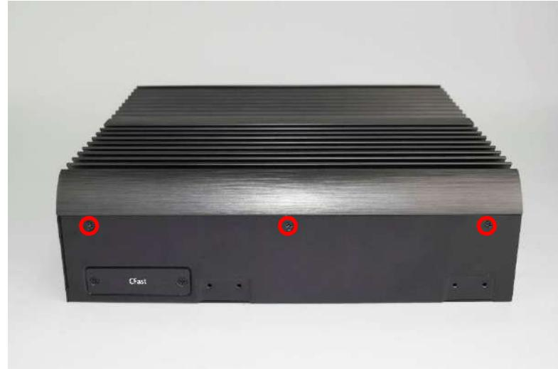
2. Unscrew the 3 screws on the bottom side.
