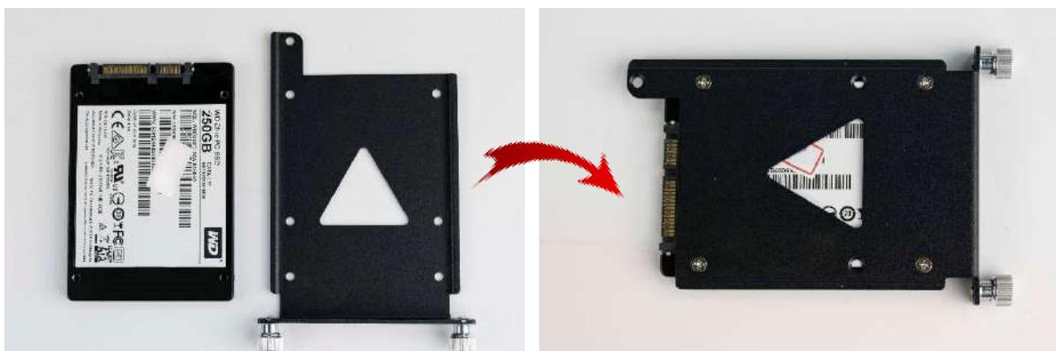
4. Slide the HDD bracket back and then fasten the sun screws.
