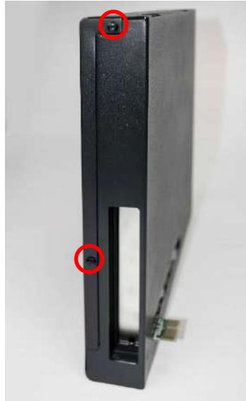
2. Push the chassis cover following the below direction to open the expansion module.
