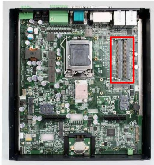
2. Insert memory module from 45 degree direction.
