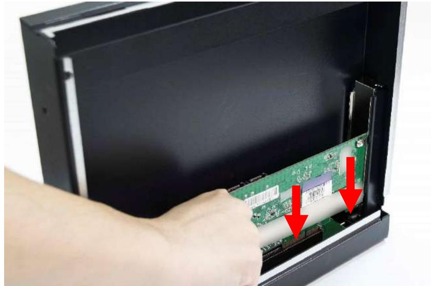
5. Install the screw back to secure the PCIe/PCI card
