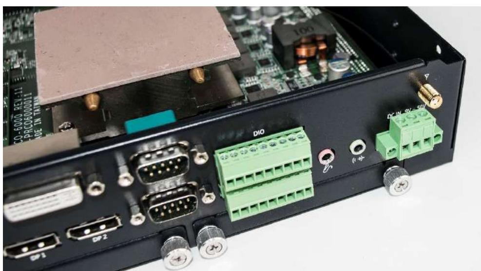
4. Put on washer and fasten the nut with antenna jack.
