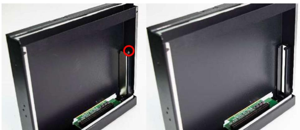
4. Insert your PCIe/PCI card into the expansion slot.
