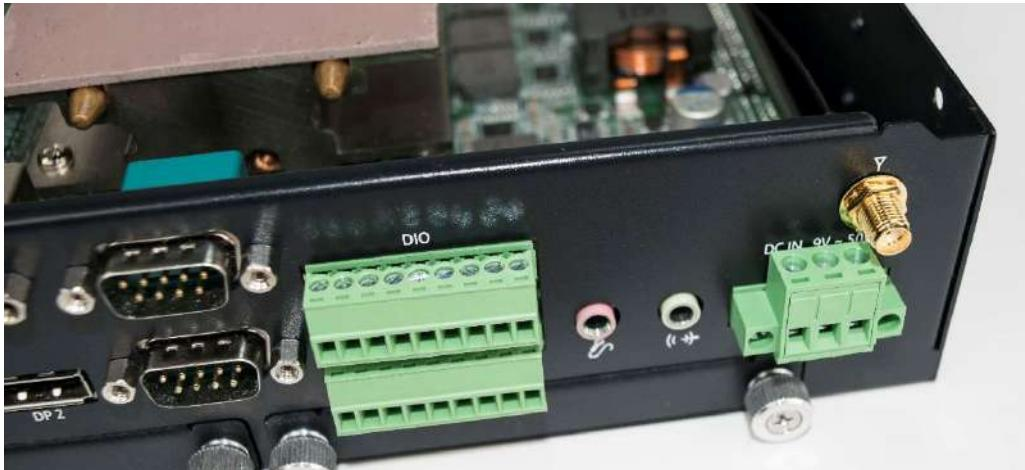
5. Assemble the antenna and antenna jack together.
