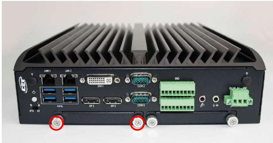
3. Lock the 2.5" HDD with HDD bracket using four screws.
