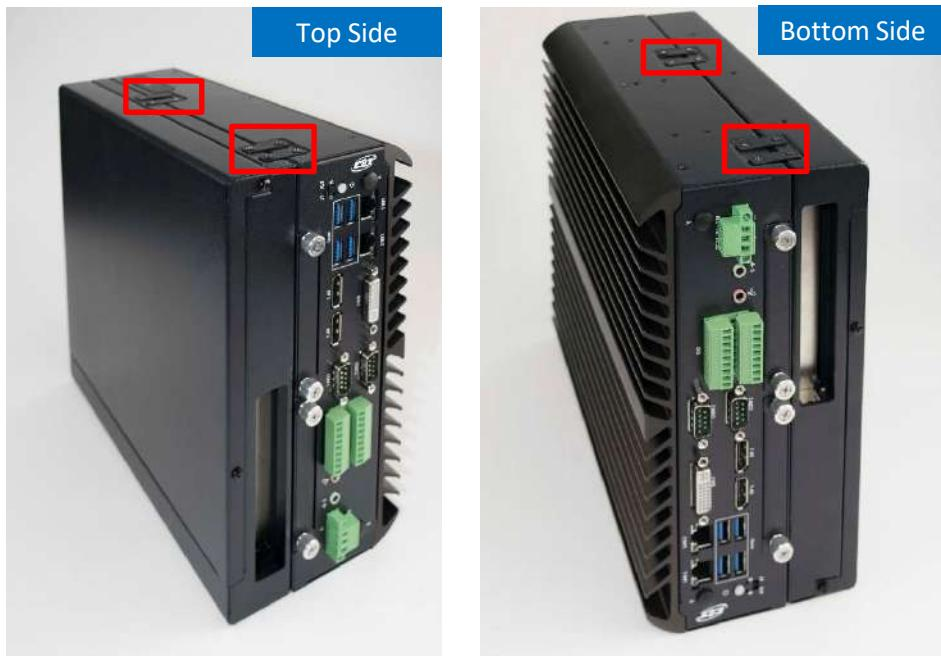
2. Now you can separate the expansion module from the computing module.
