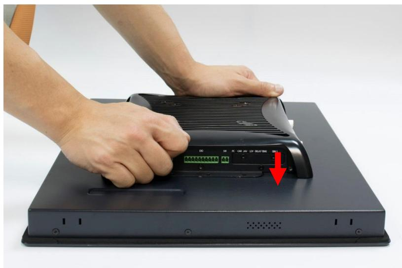
3. Lock the below 6 screws (M4x5L).
