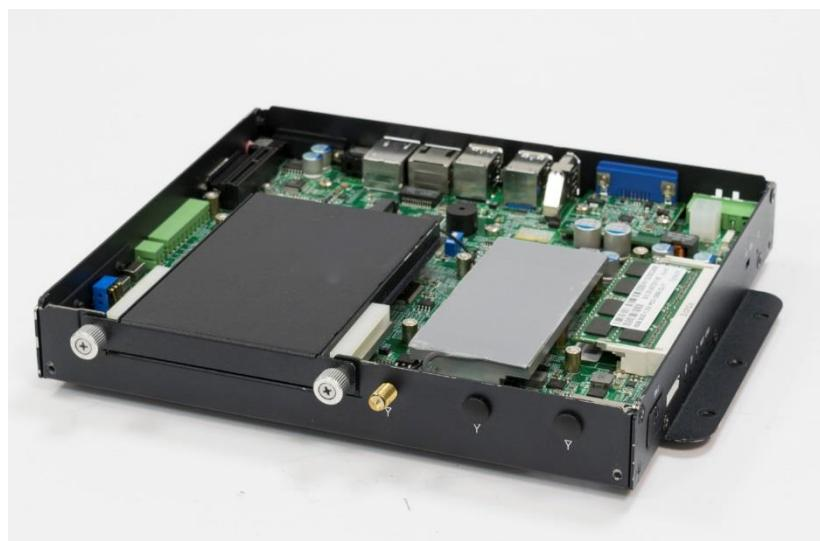
4. Put on washer and fasten the nut with antenna jack.
