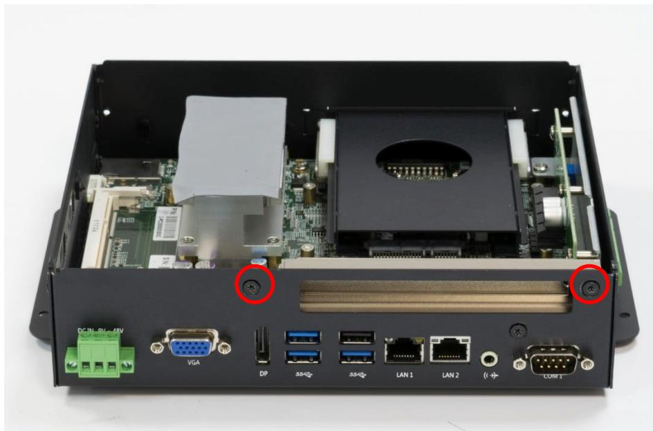
3. Lock your expansion card with the expansion window bracket by one screw (M3x5L).
