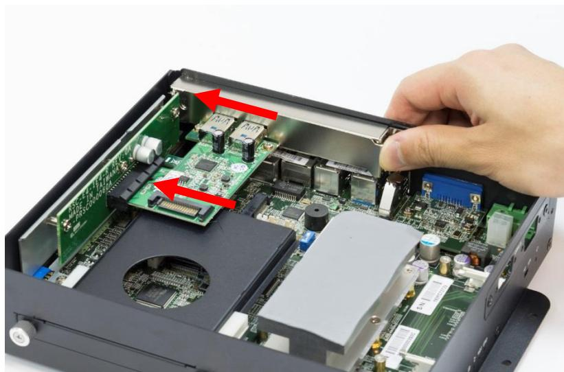
5. Fasten the two screws (M3x5L) on the panel back to lock the card and expansion window bracket.
