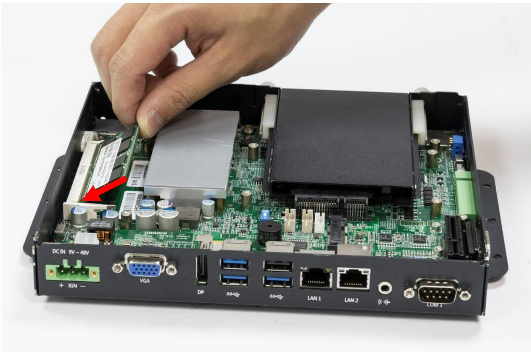
2. Press the memory module vertically downward until you hear the “click” sound. Make sure the memory module is firmly in place.
