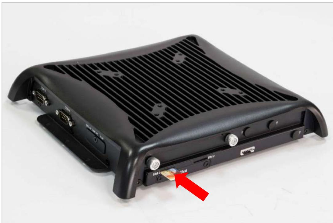
3. Please note that the installation of SIM 1 and SIM 2 has to match the installation of mini PCIe slots.
