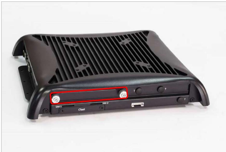
2. Unscrew the two sun screws circled below to take out the removable SATA HDD bay.
