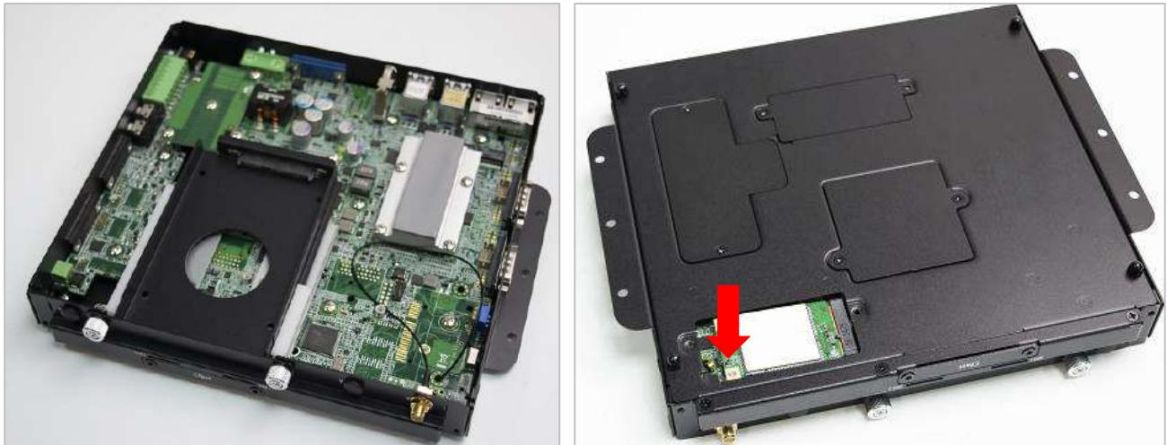
6. Assemble the antenna and antenna jack together.
