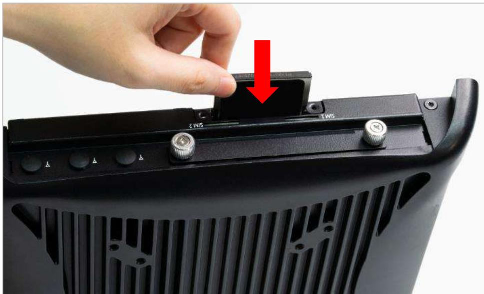
3. The socket is push-push type. Push the installed CFast card again to remove it.
