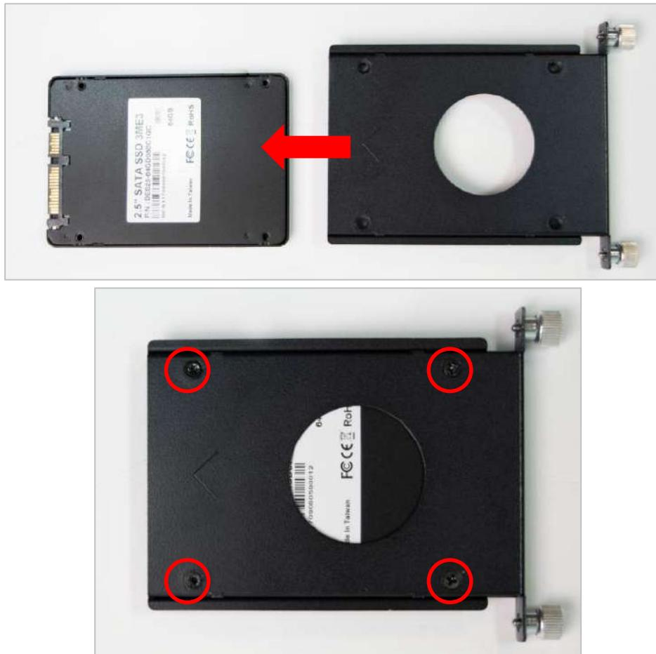
4. Slide the HDD bracket back and then fasten the sun screws.
