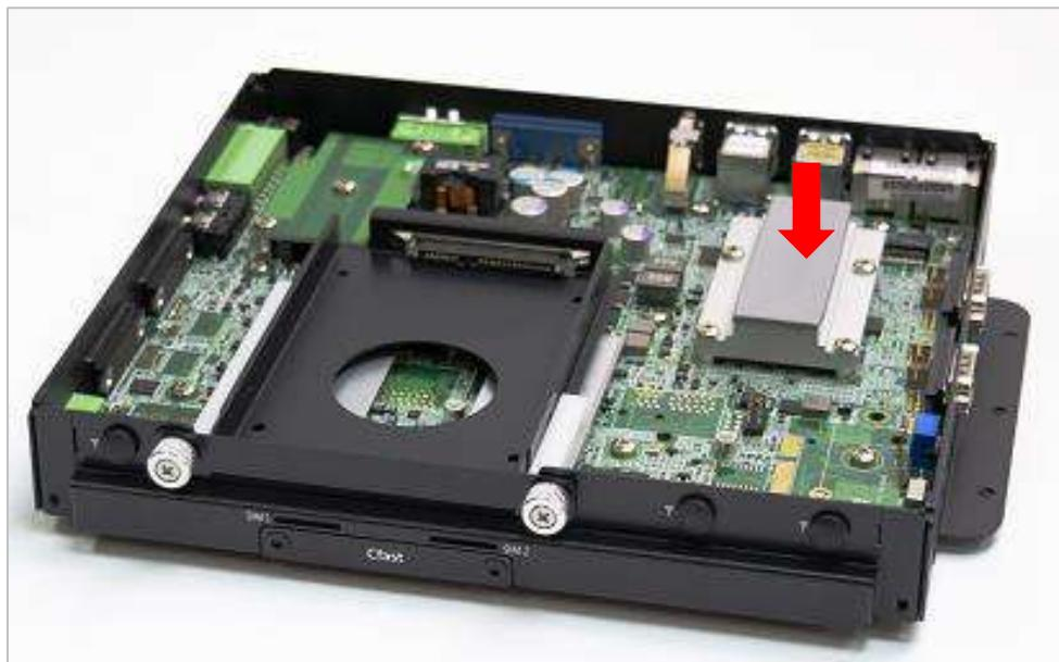
2. Close the chassis top cover following the below direction and make sure the aluminum part on the top cover is touching the thermal pad on CPU thermal block.
