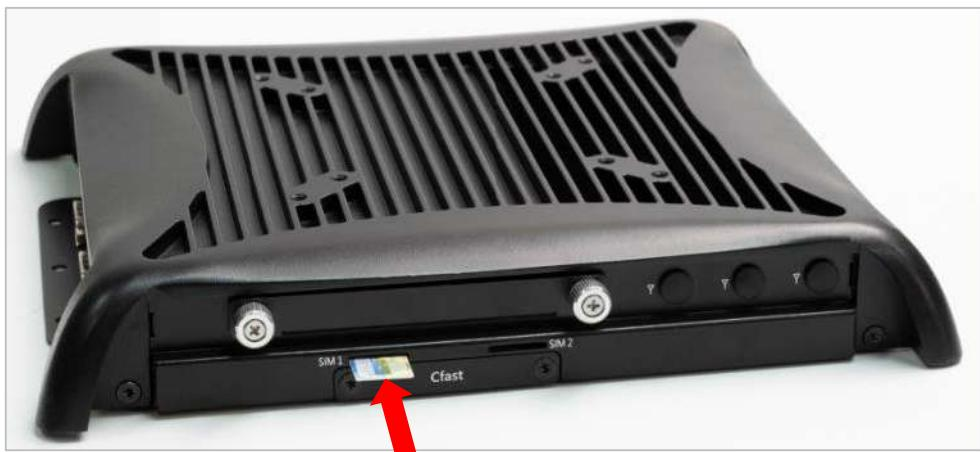
3. Please note that the installation of SIM 1 and SIM 2 has to match the installation of mini PCIe slots.
